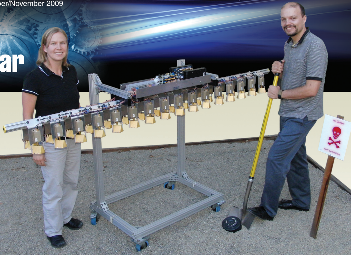
Lead engineers Christine Paulson and Kique Romero demonstrate the iRadar array at Livermore's inert mine test pit.
