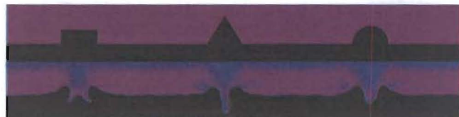
Figure 8: Demonstration run showing the ejection of material from a shocked copper surface, run on 1 CU. The sample is three-dimensional, but with a thin cross-section into the plane; only a small section of the total sample height is shown, at two different times during the simulation. (Top) Free surface prior to shock arrival. (Bottom) Initial jet formation after a shock wave has reflected from the free surface. Three different surface defects are initially present, with the same volume but different shapes, leading to different jetting patterns that will subsequently break up into ejecta particles with different size and velocity distributions.
