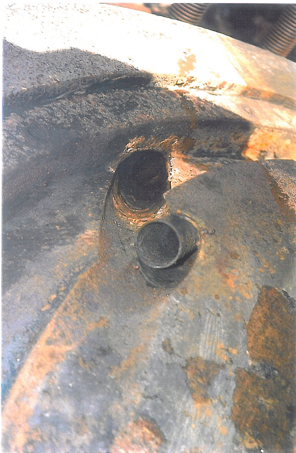
Figure 44 Nozzle Exit and End Wall After Operation
