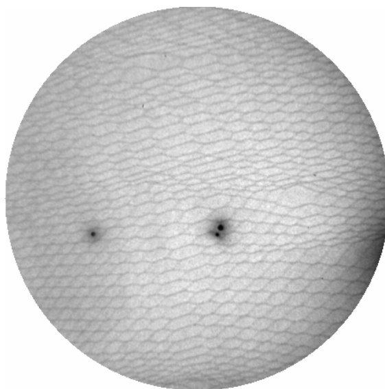
Figure 1. Bright-field LEEM image of high temperature quasicrystal surface at 905K. The electron energy is 4.4eV. The file is 1040800028. Image size, field of view (FOV) is 7 \mu m.
