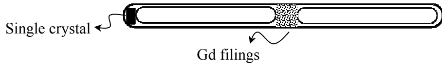
Figure 2.1. Mounting of a single crystal for high-temperature data collection
