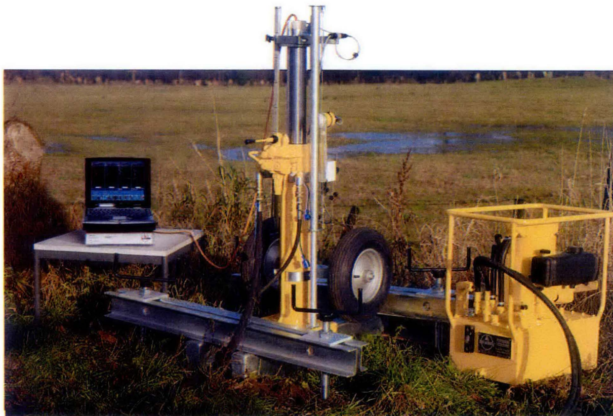
Figure 1. Hyson 100 kN Light Weight Cone Penetrometer System.
