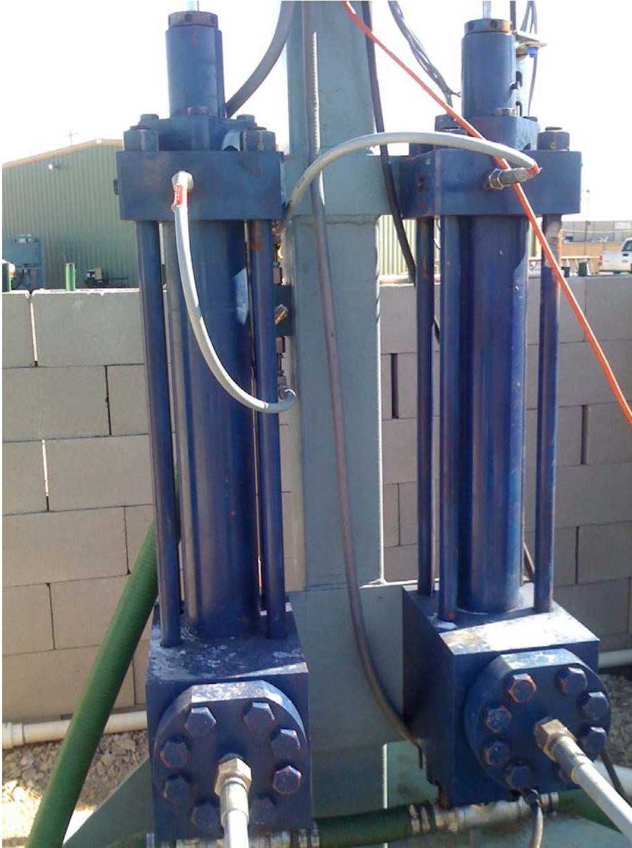
Figure 18 First Prototype High Pressure Slurry Pump (HPSP) under Test
