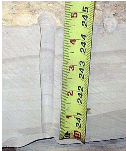
Figure 12. Hole drilled in Joachim Limestone, to a 4.5 inch depth at 4,000 psi jet pressure and 0.039 inch nozzle diameter.
