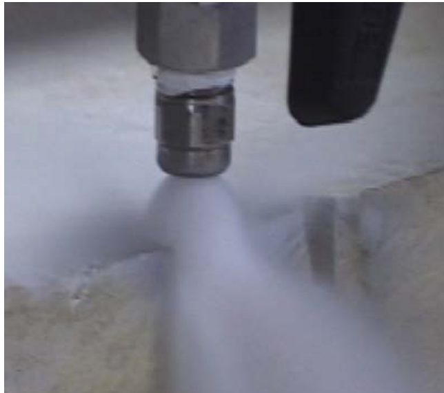
Figure 15 The use of turning vanes in a carbon dioxide feed to generate the COOAC jet.
