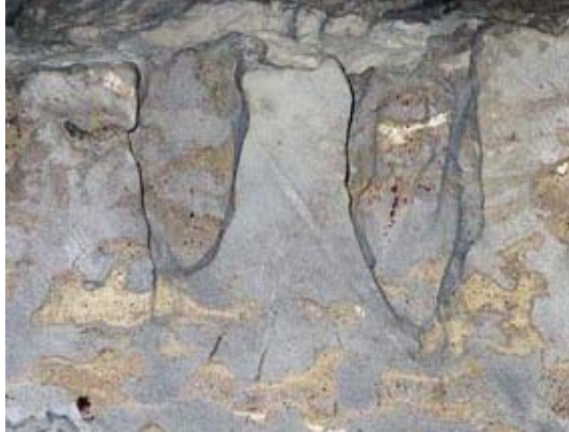
Figure 14. Holes drilled in dolomite with a diverging cone at the front of the 0.039 inch nozzle, jet pressure 4,000 psi.
