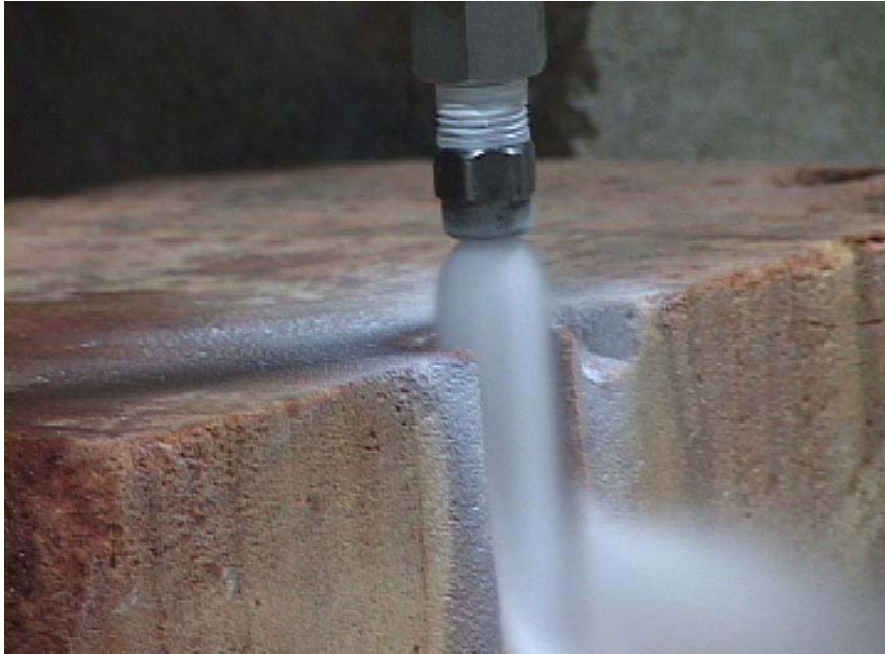
Figure 5. Carbon dioxide jet carrying abrasive and cutting into Roubideaux sandstone. The orifice diameter is 0.044 inches, jet pressure 3,000 psi, the hole diameter is 0.875 inches, and ultimate depth was 2.75 inches in four seconds.
