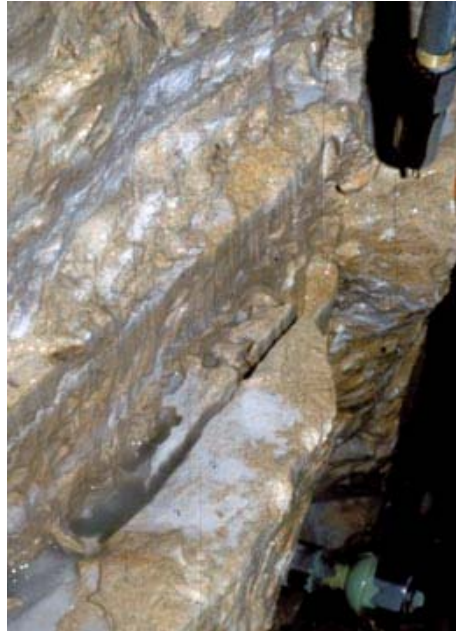
Figure 2. Slot cut through dolomite by an ASJ – although the slot is 12-inches deep it is only about 0.1-inches wide.
