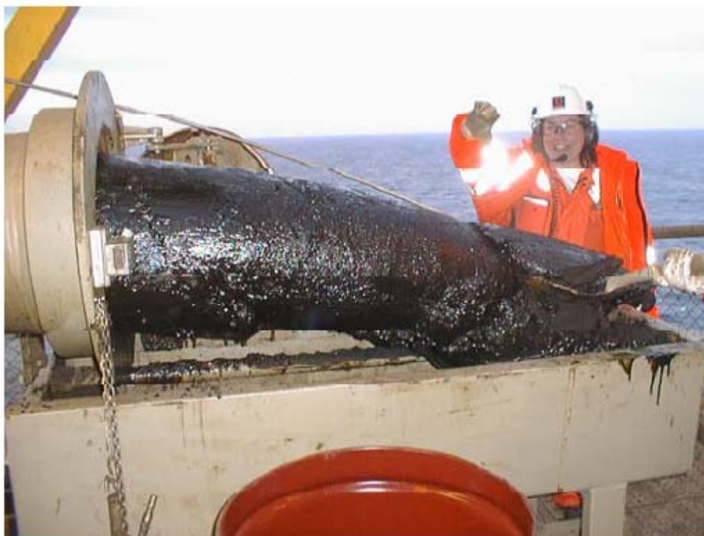
Figure 2.1: Wax plug in wellbore on platform C in North Sea (Labes-Carrier et al., 2002).
