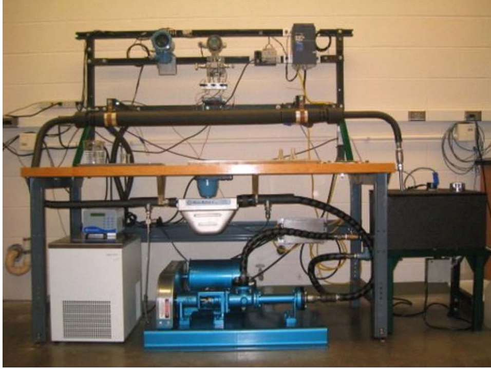
Figure 20. Photo of Fully Assembled Flow Loop
