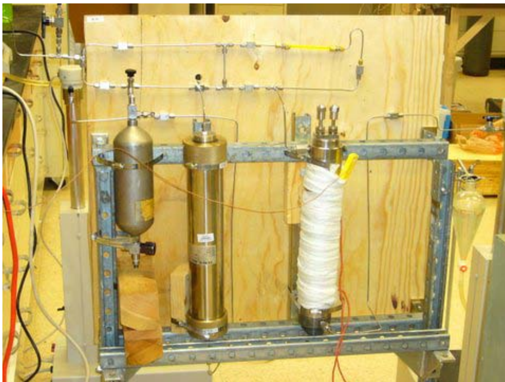
Figure 4.6.2: Laboratory setup for GOR measurement.
