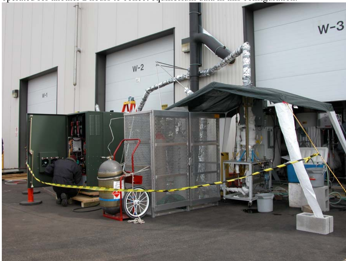
Figure 3 Setup in the parking lot at INEEL. Acumentrics fuel cell at left, SOFCo reformer at right. Natural gas supply in tank with wheels, the insulated line at the top is for the steam supply.
