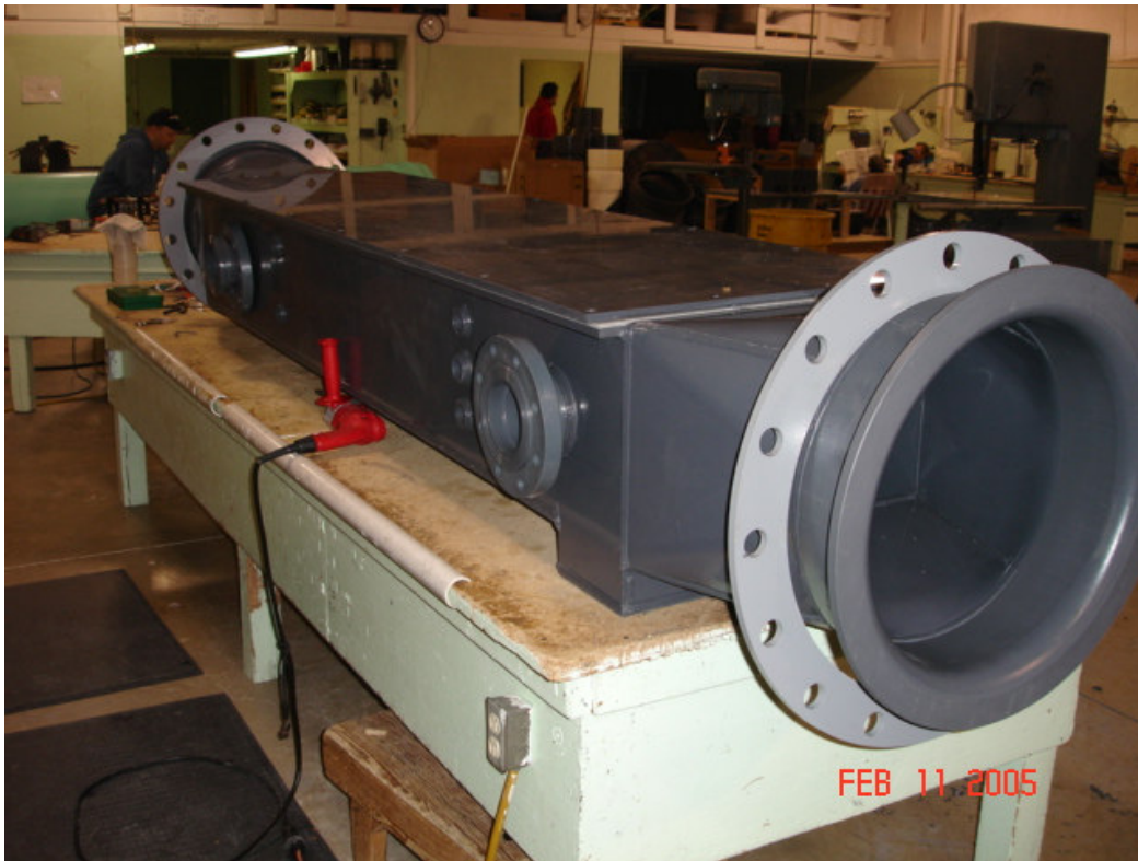
Figure 3-11. Wet MerCAP™ Housing for Installation at Plant Yates
