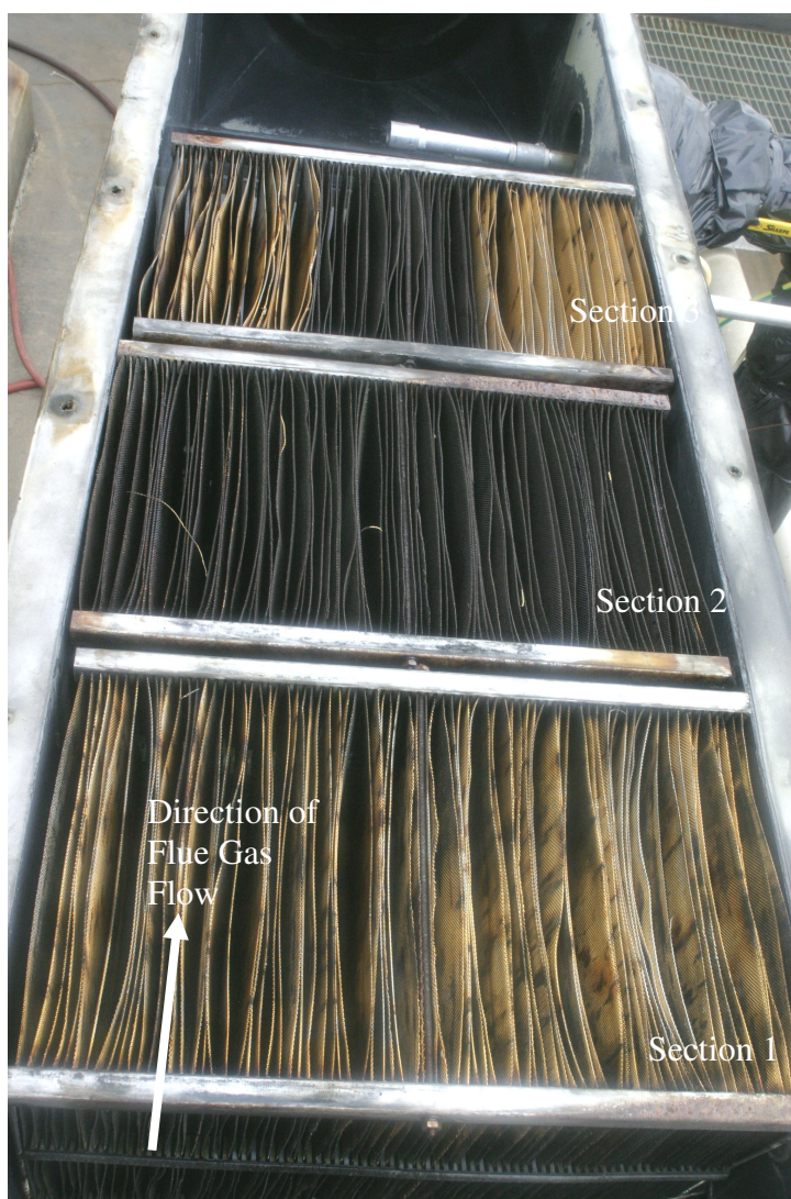
Figure 4-29. Gold Substrates after One Month of Flue Gas Service (2006 test).
