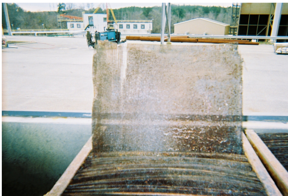
Figure 4-20. Corroded Gold Screens in the MerCAP™ Reactor
