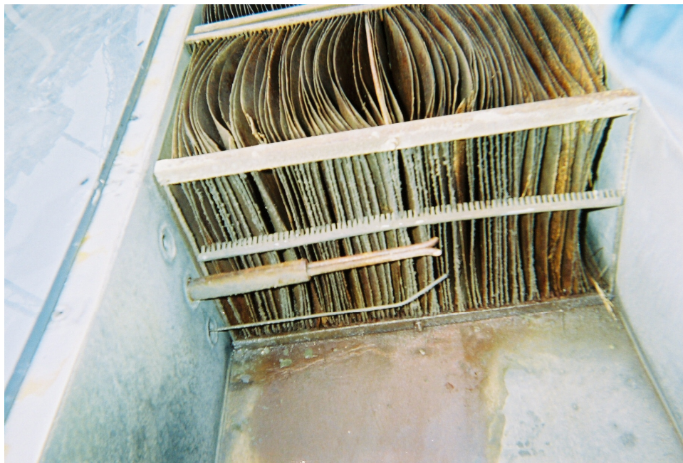
Figure 4-19. Corroded Gold Screens in the MerCAP™ Reactor Following Flue Gas Flow Reversal.
