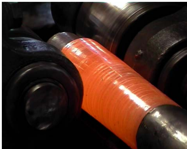
Figure 6 Hot rotary cross-rolling of ODS MA956 tubes
