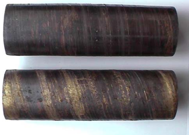
Figure 7 Surface markings on ODS MA956 tubes cross rolled at oblique \beta=2^\circ (top) and \beta=8^\circ (bottom).
