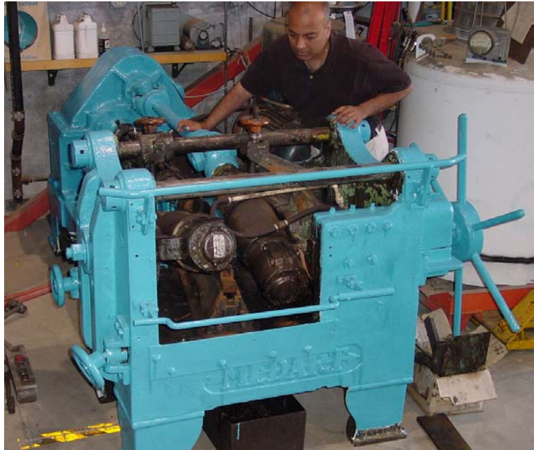
Figure 5 Cross-Rolling equipment currently installed at UCSD. The equipment is capable of rolling up to 1-1/2" bar/rod and up to 2-1/2" diameter alloy tubing in a continuous fashion
