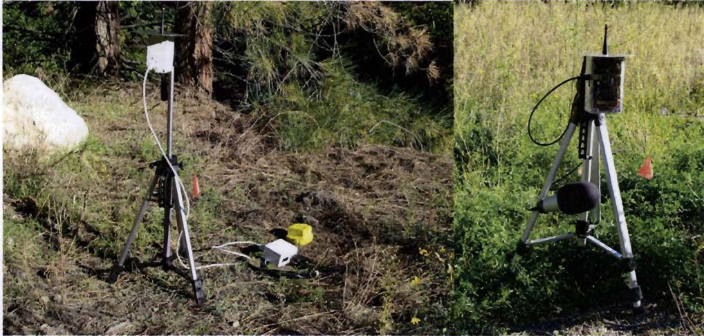
Figure 1 Mica2 mote, signal conditioning box, seismic sensor (left). Stargate and acoustic sensor (right)
