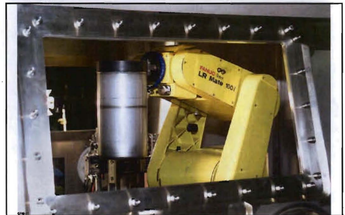
Figure 7. Handling the welded 3013 can.
