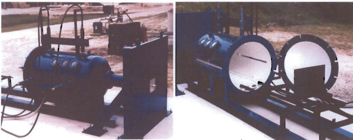
Fig. 3. Two views of the NASA-funded inhibited shaped charge launcher located at Southwest Research Institute in San Antonio, Texas. The evacuated flight and target chamber is the main component. The large cables are attached to the x-ray heads used for in-flight diagnostics. The conical charge liner completes the vacuum seal; in the left image it has been placed on the blast shield for reference.
