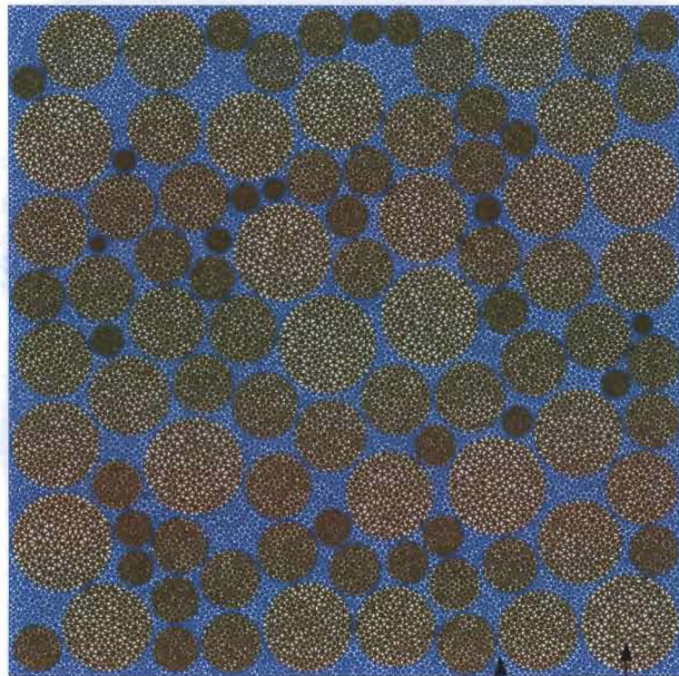
RVE for PBX9501 (77%HMX+23%DB)
