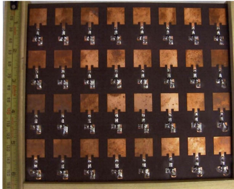
Figure 7. Thirty-two element, 5.8 GHz rectenna array designed at LANL
