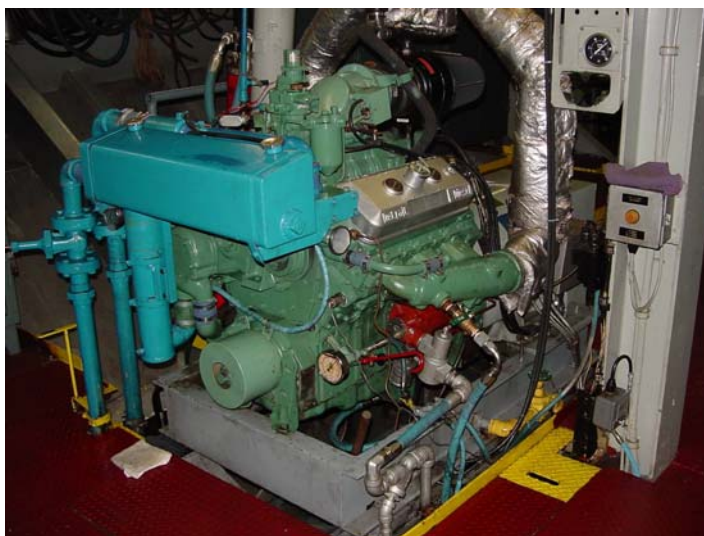
Figure 14. M/V Issaquah vessel service engine, Detroit Series 60 DDEC.
