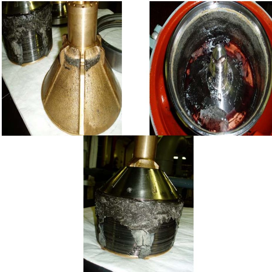
Figure 20. M/V Issaquah with abnormal sludge buildup in fuel purifier.
