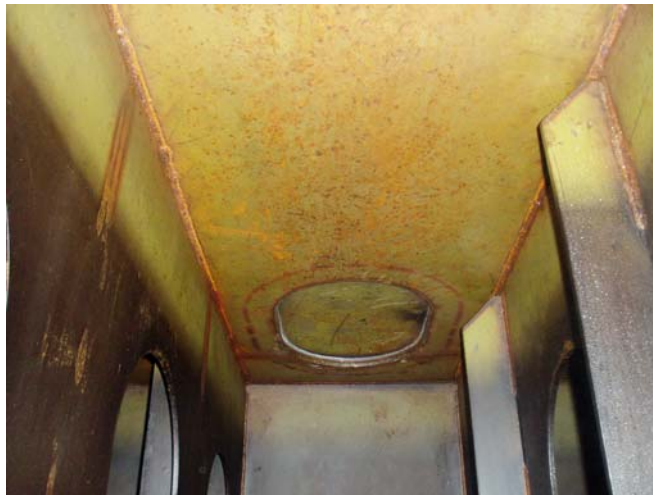
Figure 12. Vessel deep fuel tank after B100 hand wipe down.
