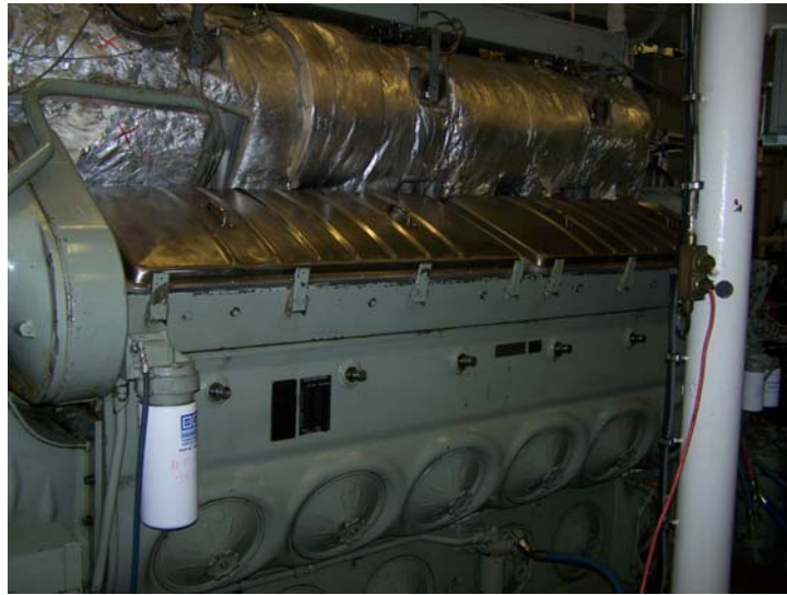
Figure 16. M/V Klahowya / Tillikum main propulsion engine EMD 12-645-F7B.
