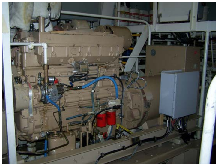
Figure 17. M/V Klahowya/Tillikum vessels service engine Cummins NTA 855.
