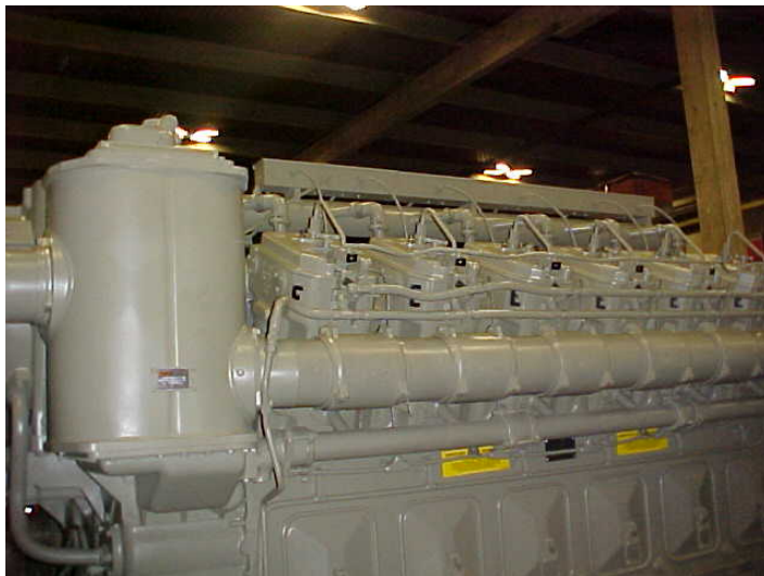
Figure 13. M/V Issaquah main propulsion engine, GE 7 FDM 12 EFI.
