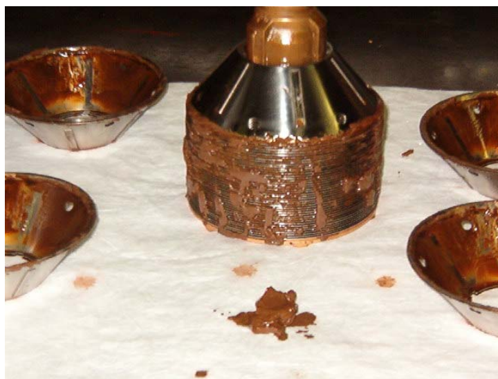
Figure 18. Fuel purifier disk stack with "butterscotch mousse".
