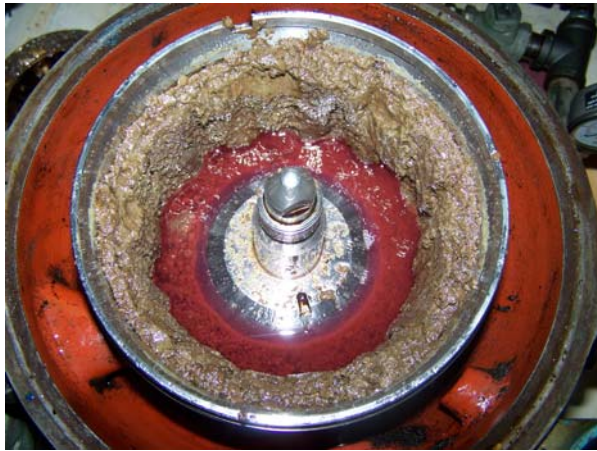
Figure 22. Oil purifier without Biobor.
