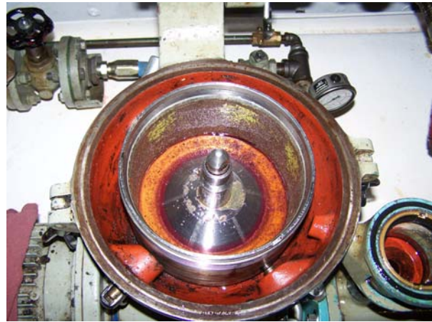
Figure 23. Oil purifier w/3 treatments of Biobor.
