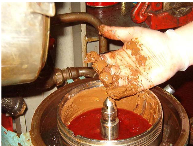
Figure 4. Fuel purifier sludge from 2004 biodiesel pilot tests.
