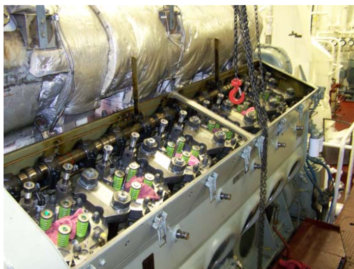
Figure 15. M/V Tillikum main propulsion engine shown with fuel injectors removed (rags in place).
