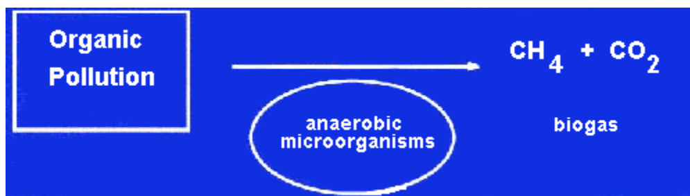
Figure 3-9. Anaerobic Decomposition of Organic Material
