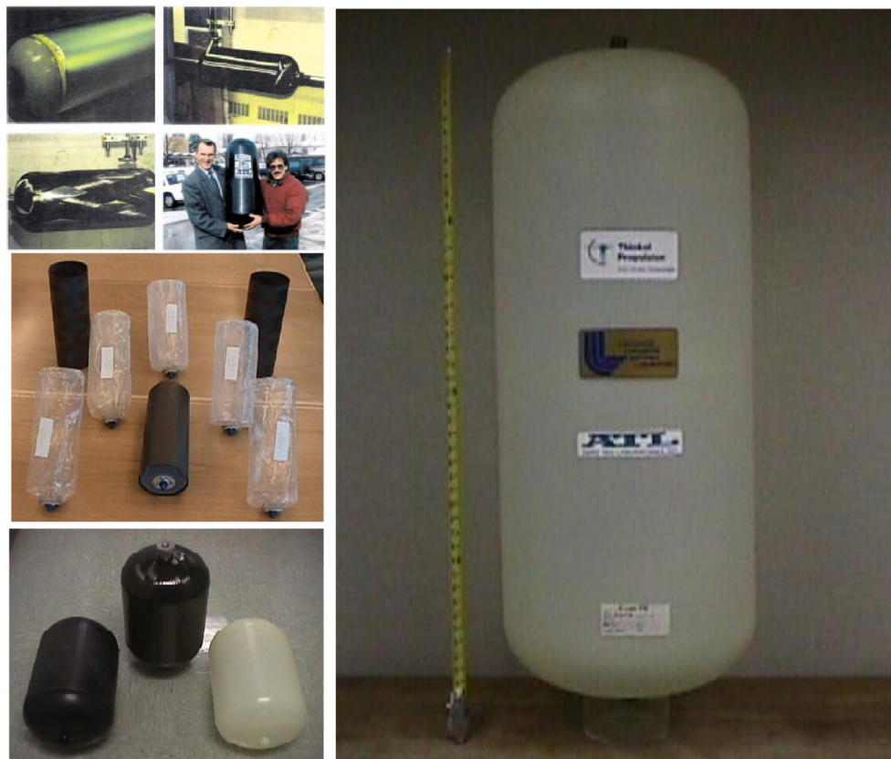
Figure 10 - Photos of LLNL/Thiokol/ATL Bladders and Tanks
