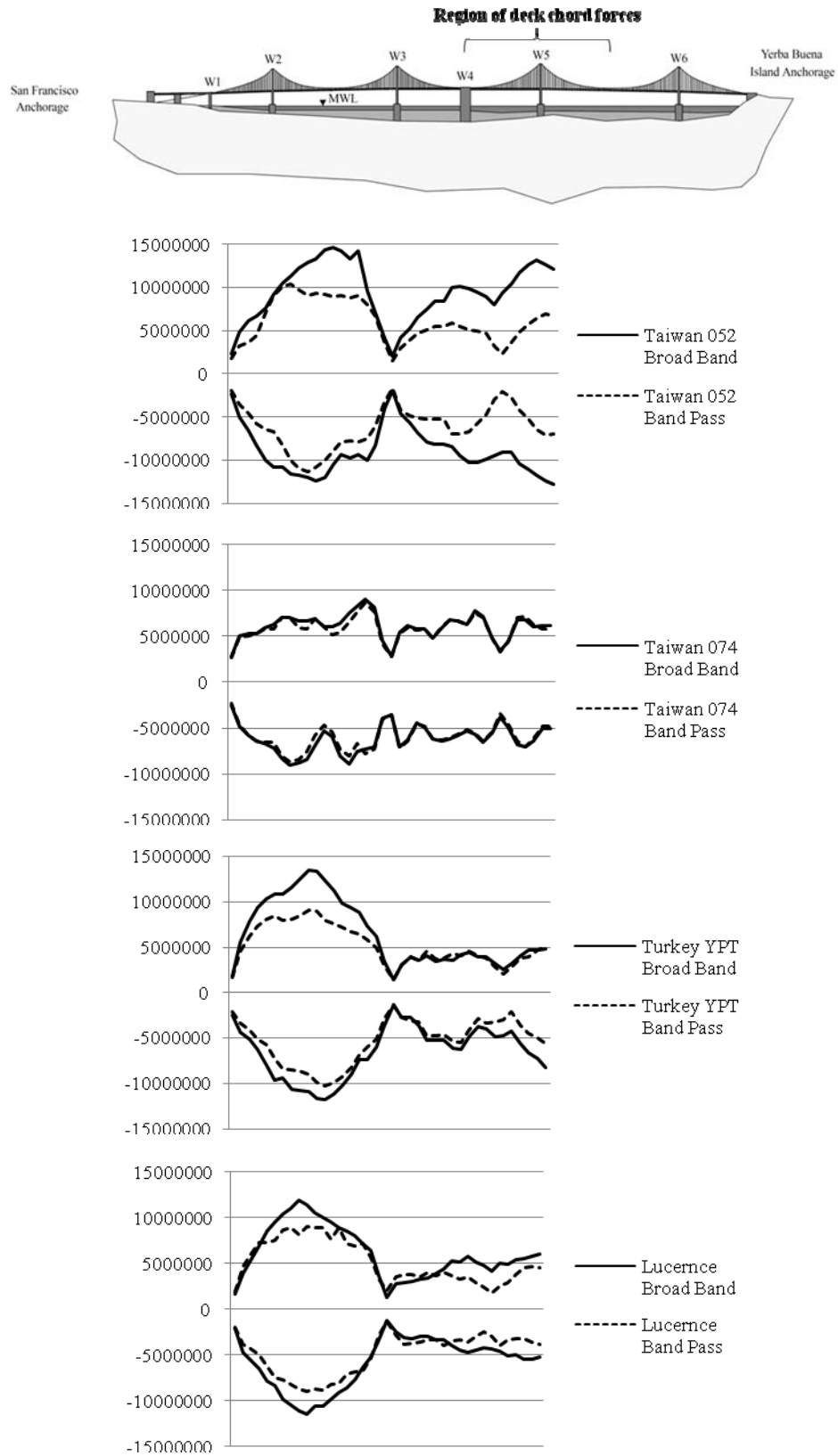
Figure 8. Envelope of stiffening truss chord forces (nt) for broad-band and band-passed near-fault motions
