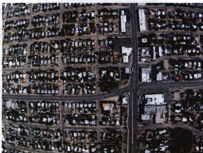
Figure 1. This shows an uncorrected frame of the original imagery taken from the helicopter hovering over Tucson. The radial distortion is clearly evidenced by the curved streets.
