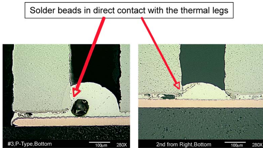
Figure 9. Optical images show the solder beads in direct contact with the side of the P leg on the sideways.
