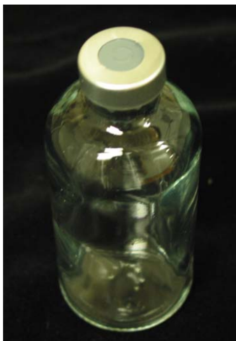
Figure 2. Seventy ml Wheaton vial with grey butyl stopper secured by an aluminum cap.
