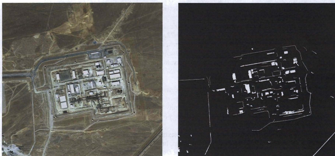
Figure 7. An example of man-made object detection using partitions on single LODs of the built hierarchy. Left: Image of nuclear facility at Arak, Iran. Source: DigitalGlobe.com. Right: the result of detection (in white). In order to achieve better detection it is necessary to perform the detection across multiple LODs and then integrate results.
