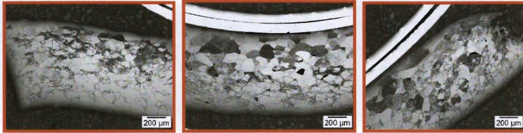
Figure 3. Optical metallography of twins and slip bands in Ta as a function of position relative to the HE side-interface initiated sample. Photos coincident with the left, center, and right locations indicated in Fig. 2.
