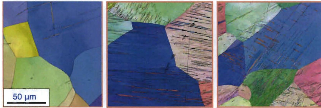
Figure 4. EBSD maps showing twins in Ta as a function of position relative to the HE initiation site for the side interface initiated sample. Photos coincident with the left, center, and right locations indicated in Fig. 2.
