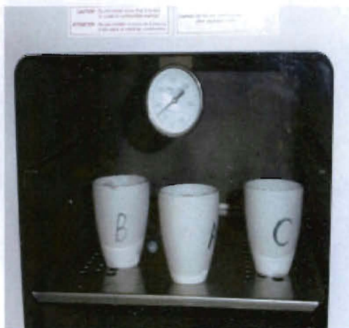
Figure 4.2: Crucibles with foam material are drying in the vacuum oven at the same time.
