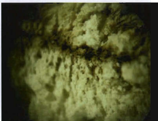
Figure 5.7: Post-combusted \text{Y}_2\text{O}_3\text{:Bi} nanopowder with glycine fuel at 10X magnification.
