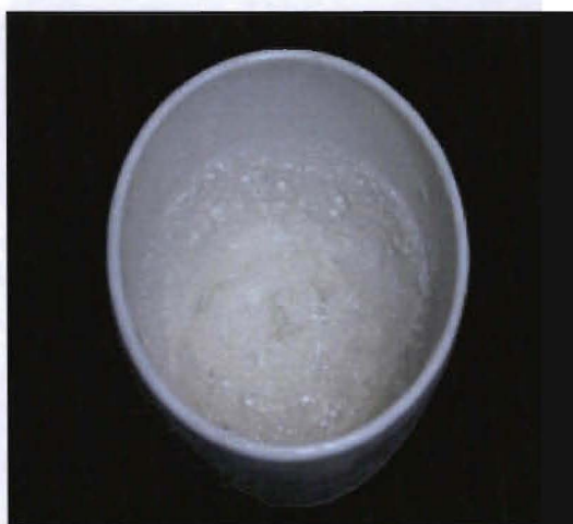
Figure 4.3: Pre-combustion material after drying in a vacuum oven.
