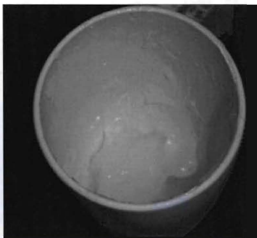
Figure 4.1: Foam produced by reacting yttrium nitrate, bismuth nitrate, and glycine.
