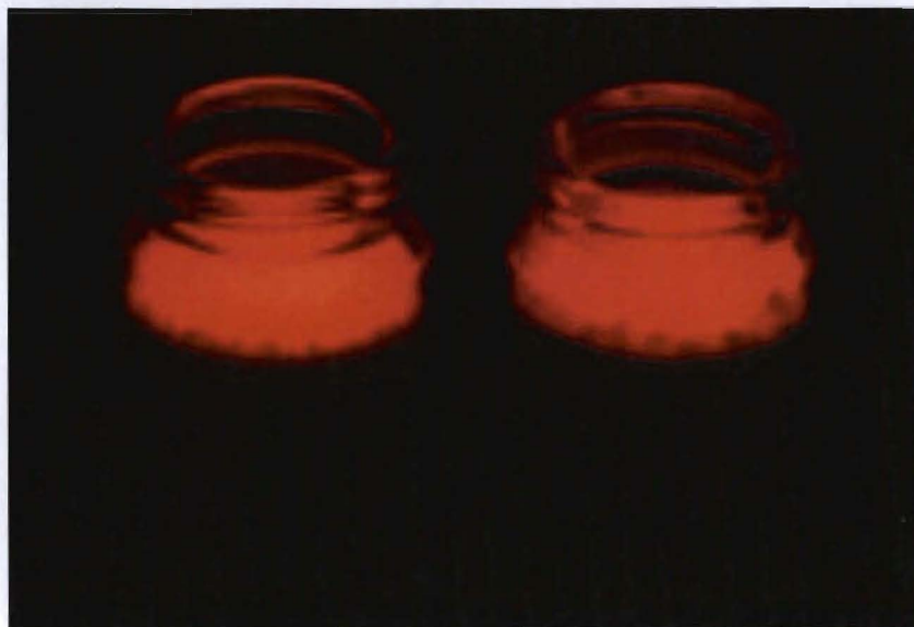
Figure 2.8: Luminescence of \text{Gd}_2\text{O}_3\text{:Eu} nanophosphors under UV excitation.
