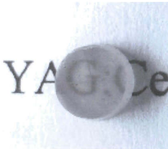
Figure 2.4: \text{Y}_3\text{Al}_5\text{O}_{12}:\text{Ce} consolidated nanoceramic [14].
