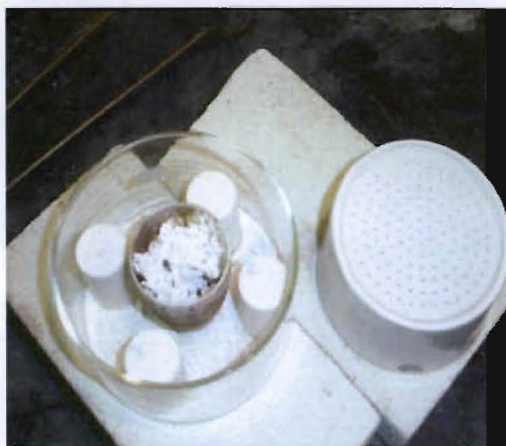
Figure 4.4: Apparatus utilized for combustion of the nanophosphors consists of a Pyrex crystallization dish with four alumina tubes (left). During combustion a ceramic dish (right) is placed atop the alumina tubes to contain the combusted material.
