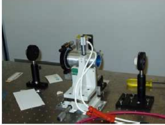
FIG. 3.4: A Pockels Cell between two linear polarizers.
