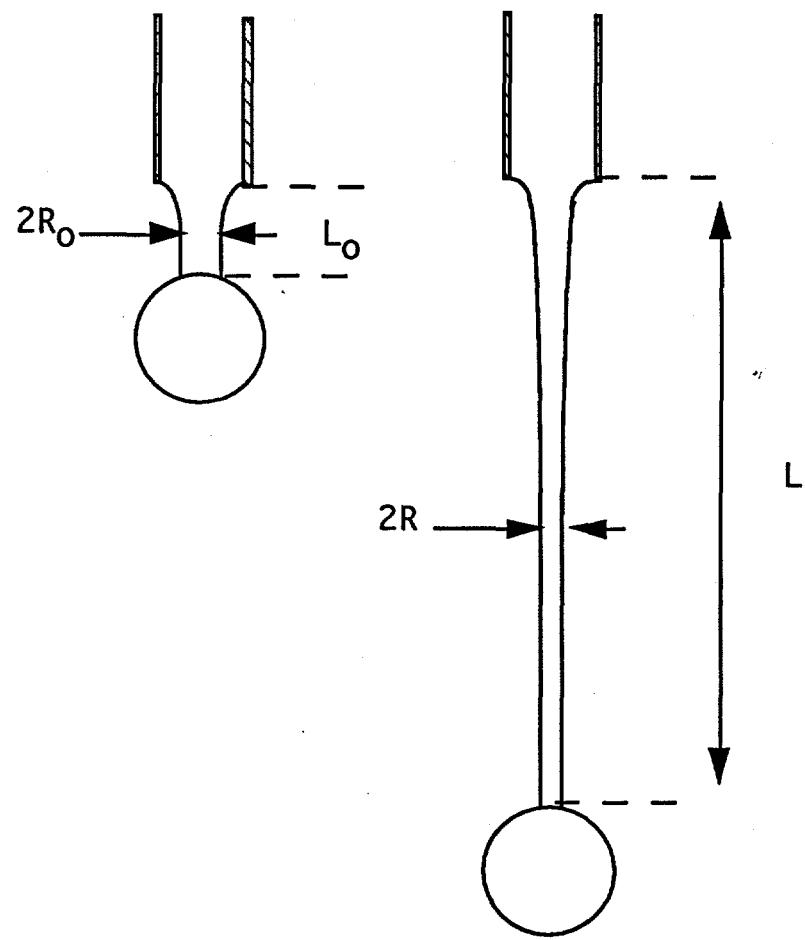
Fig. 2 Homogeneous Extension of Liquid Ligaments
