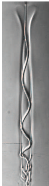
Figure 3: The density jet descending in a density-stratified fluid.
