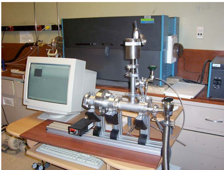
Fig. 6. Facility for leak testing and continuous monitoring of SOFC seals both at room temperature and up to 1200°C under a variety of pressure drops.
