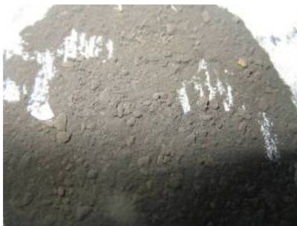
Figure 53: Photograph of CeN powder produced via a carbothermic reduction prior to nitridation of a \text{CeO}_2 and carbon powder mixture. The thermal processing was carried out at a maximum temperature of 1400^\circ\text{C} .
