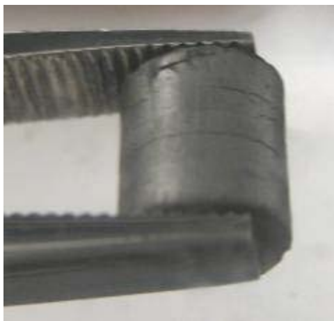
Figure 88: 68%TD sintered UN pellet after cold pressing wet-milled UN (in toluene with zinc stearate and PVB) at 300 MPa. The 45%TD green pellet was sintered in very pure argon at 1500°C for 10 hours.
