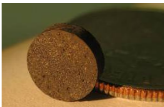
Figure 91: UN pellet sintered at 1550°C for 5 hours in very pure argon using as-synthesized powder (i.e. no milling, binder, or lubricant). The pellet was pressed at 420 MPa to 56%TD and only reached a sintered density of 61%TD.
