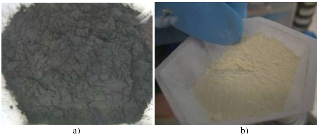
Figure 51: a) Photograph of glassy carbon spherical powder and b) Photograph of CeO 2 powder prior to being mixed together to initiate the carbothermic reduction prior to nitridation synthesis route to produce CeN.
