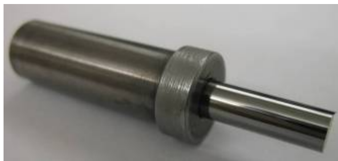
Figure 87: Photograph of a 0.2500" diameter carbide pellet die and pellet punch used for pressing UN pellets.
