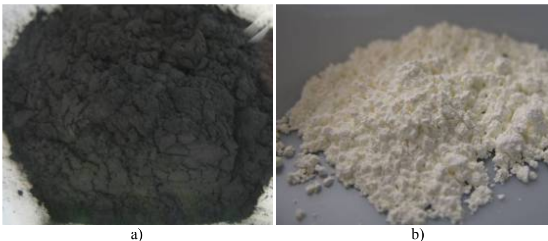
Figure 30: The starting materials of the carbothermic reduction prior to nitridation synthesis route to produce DyN are a) Glassy carbon spherical powder mixed with b) \text{Dy}_2\text{O}_3 powder.
