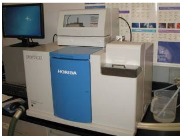
Figure 6: Photograph of a Horiba LA-950 Laser Diffraction Particle Size Analyzer for use in characterizing powder particle size, including powders from: Commercial vendors, those synthesized in the planetary ball mill, or those synthesized by conventional furnace techniques for sintering studies.
