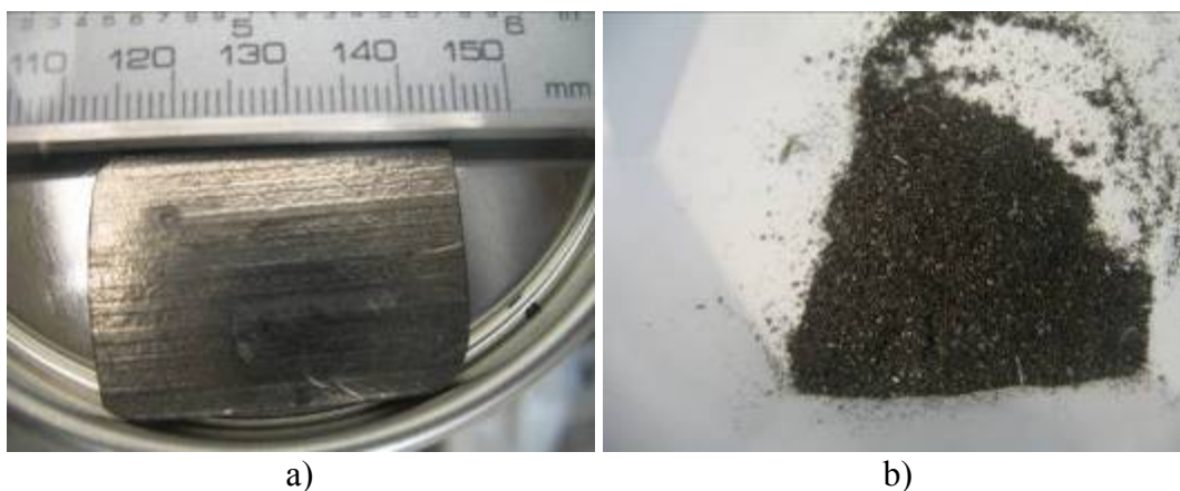
Figure 19: Shown are the starting materials for the ball-milling synthesis route of uranium nitride at room temperature including (a) a uranium metal ingot obtained from the Idaho National Laboratories and (b) uranium metal flakes obtained from flake the metal ingot with a carbon-steel file.
