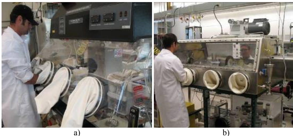
Figure 1: Two argon filled gloveboxes for material handling and storage. Figure a) shows the Plas-Lab closed loop containment isolator glove box for sample preparation and storage. The Plas-Lab glovebox also contains a hydraulic press and balance. Figure b) shows the heavy-duty stainless steel glovebox containing a 1200°C tube furnace for low temperature hydrogen synthesis routes.
