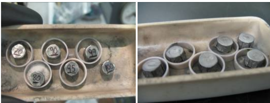
Figure 99: Photographs of the (U, Dy)N pellets encapsulated in Nb foil before and after a typical sintering profile in Ar – 1%N 2 .
