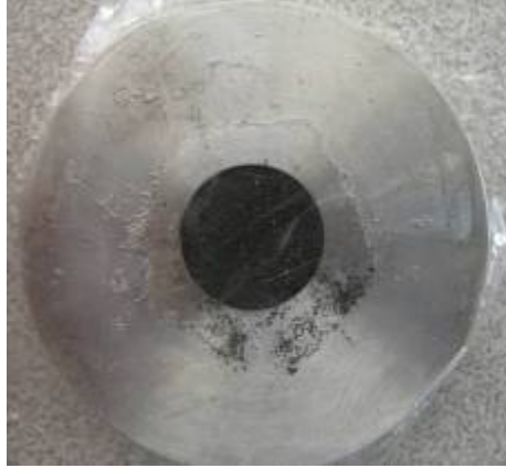
Figure 13: Stainless steel sample holder used for obtaining XRD patterns. The powder sample is placed and leveled in the center (10 mm diameter) and covered with an x-ray transparent film to temporarily protect it from oxidation during transportation to and during XRD analysis.
