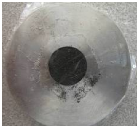
Figure 40: Stainless steel sample holder used for obtaining XRD patterns. The powder sample is placed and leveled in the center (10 mm diameter by 1 mm deep) and covered with an x-ray transparent film to temporarily protect it from oxidation during transportation to and during XRD analysis.
