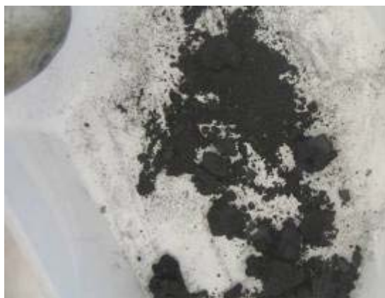
Figure 17: Photograph of UN synthesized via a hydride prior to nitridation of pure uranium metal pieces in pure H_2 prior to pure N_2 at 320^\circ C and a pure argon gas at 1375^\circ C .
