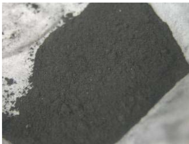
Figure 32: DyN powder produced via a carbothermic reduction prior to nitridation of a \text{Dy}_2\text{O}_3 and carbon powder mixture at 1500^\circ\text{C} .
