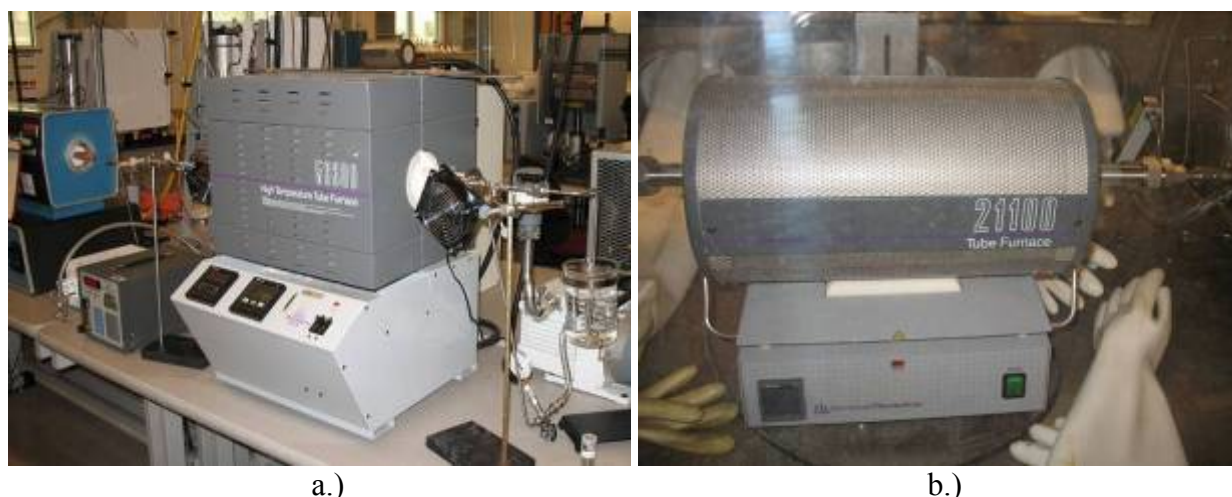
Figure 3: Furnaces in the Advanced Materials Laboratory for processing nitrides. a) Photograph of a high temperature Thermolyne 59300 tube furnace equipped with oxygen and moisture-gettering capabilities. b.) Photograph of a Barnstead Thermolyne 21100 tube furnace for low temperature hydrogen processes. The Barnstead tube furnace is located in an inert atmosphere glovebox to allow oxygen sensitive sample insertion and removal.
