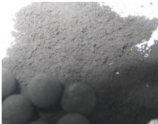
Figure 22: Photograph of the uranium nitride formed from ball-milling the flakes for 24 hours at room temperature in a nitrogen atmosphere.
