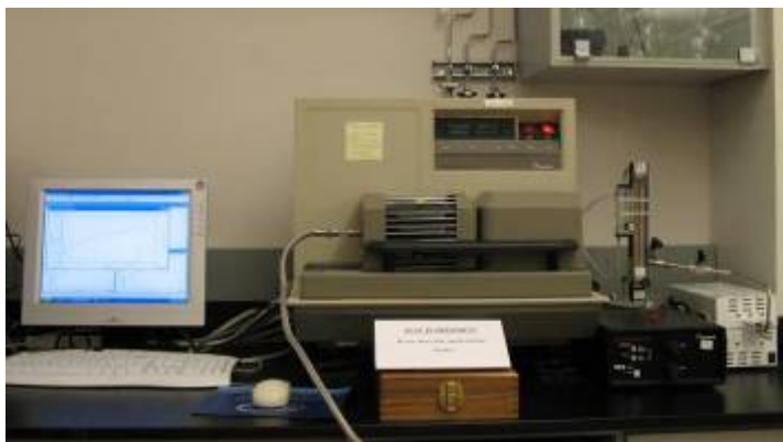
Figure 9: Photograph of TA Instruments SDT 2960 Simultaneous DSC/TGA that is used to study the oxidation kinetics of the nitride powders. This instrument is capable of reaching 1000°C in 10 minutes and 1500°C in 30 minutes with 1°C accuracy and can record DSC, DTA, and TGA data.
