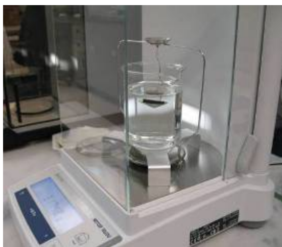
Figure 8: Photograph of the Mettler Toledo scale with the immersion density measurement kit attached. The kit provides immersion weights that, using Archimedes' principle, can be correlated to the density of nitride fuel pellet.
