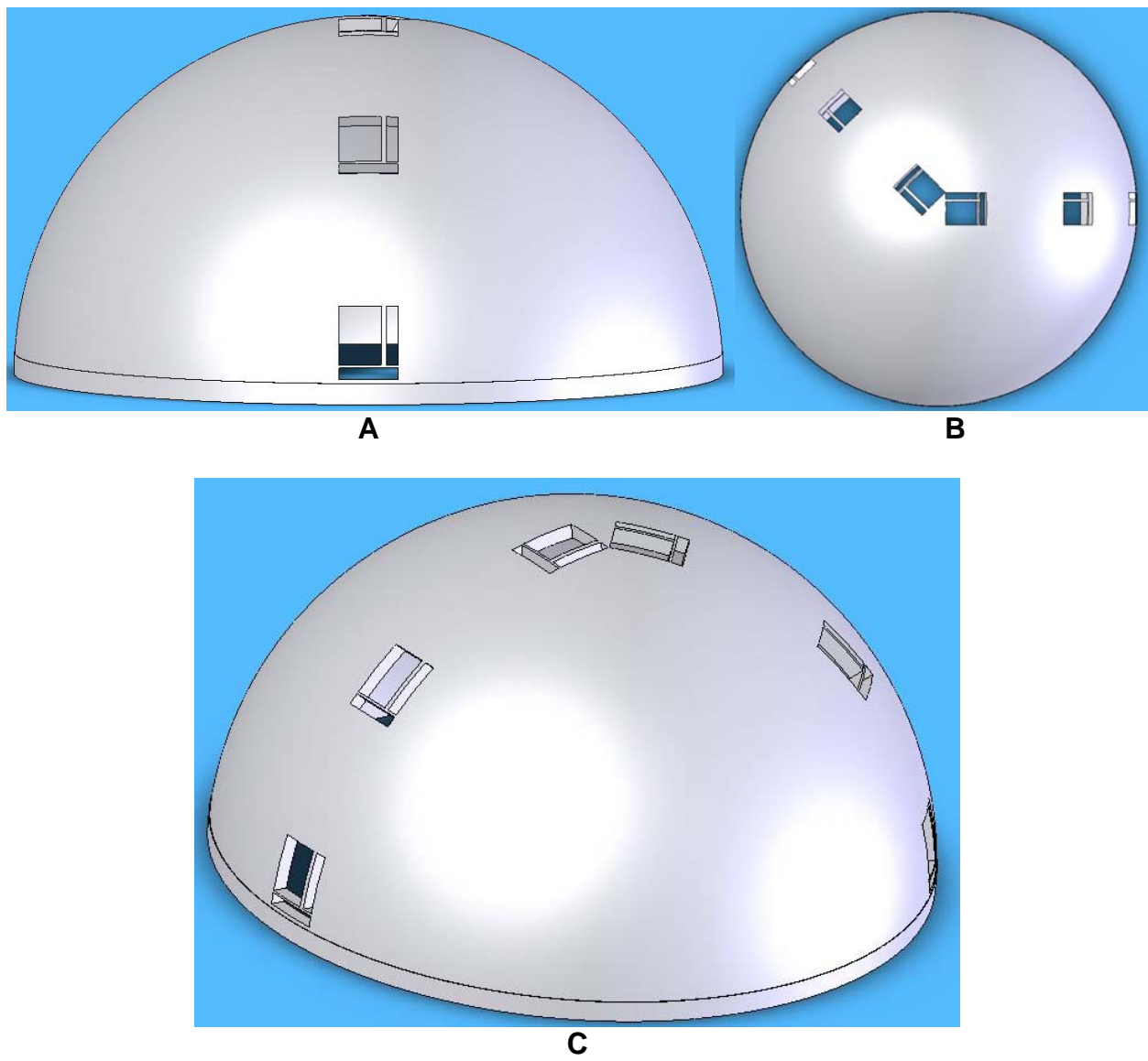
Figure 6 Locations of metallographic (hardness) and tensile samples for hemishells of 21-6-9 stainless steel, Ta-2.5% W, and pure vanadium. Large rectangles represent metallographic and hardness samples. Slender rectangles are tensile bar locations. Side view is shown in A, top view in B, and trimetric in C.
