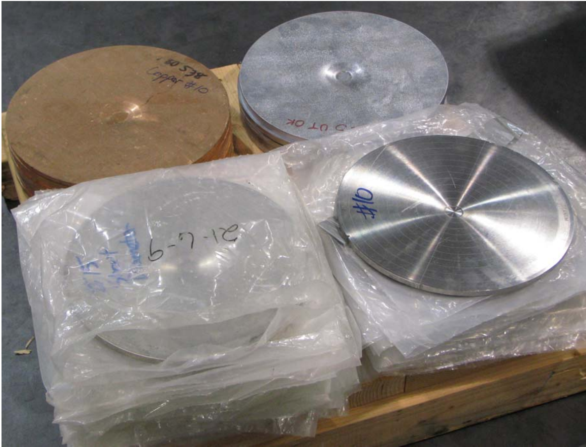
Figure 1 Pre-forms of the four materials: copper (upper left), vanadium (upper right), 21-6-9 stainless (lower left), titanium alloy (lower right).
