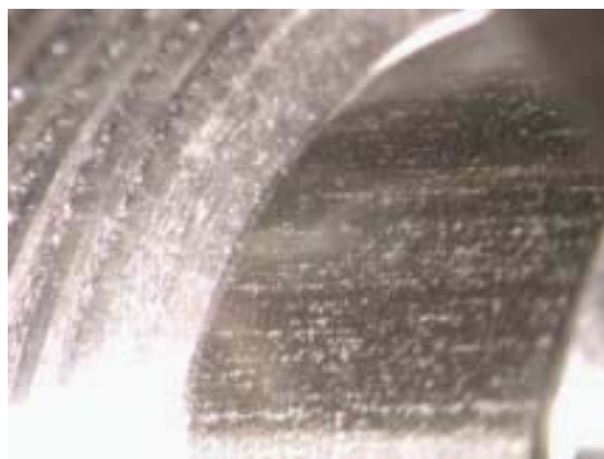
Figure 3: White Spots from Passivation
