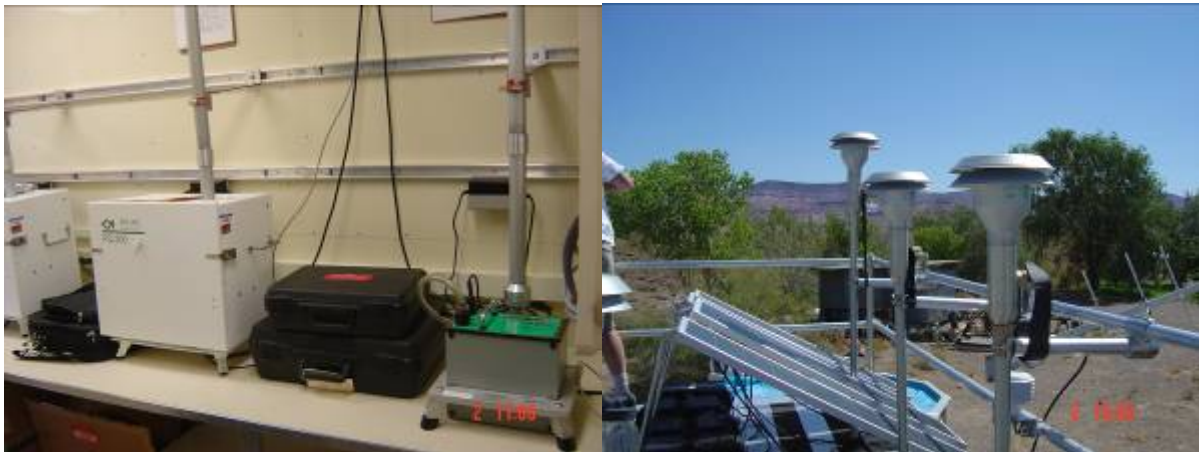
Figure 2. Photographs of PQ100 (green/gray box in left photo), PQ200 (white box in left photo) and their sampling inlets (right photo).
