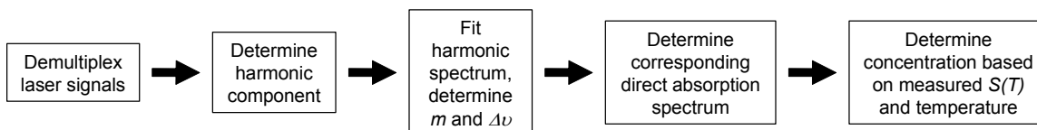
Figure 1: Measurement process based on application of theoretical developments to WMS for highly accurate, time-resolved concentration determination.
