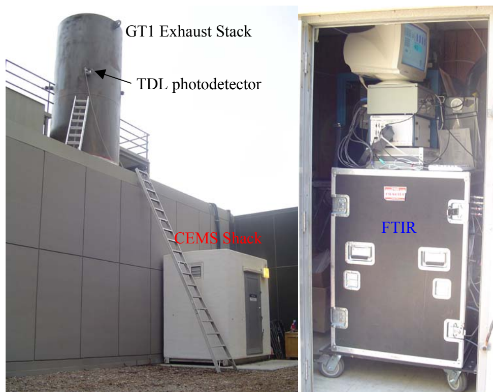
Figure 3.19: Left: GT1 exhaust stack and CEMS shack; Right: TDL system on top of FTIR
