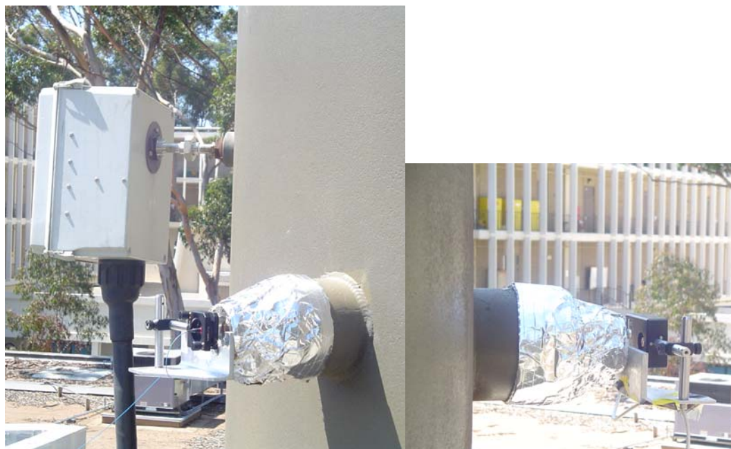
Figure 3.20: Left: TDL collimating lens window assembly (note the CEMS sample hose in the background); Right: TDL photodetector window assembly
