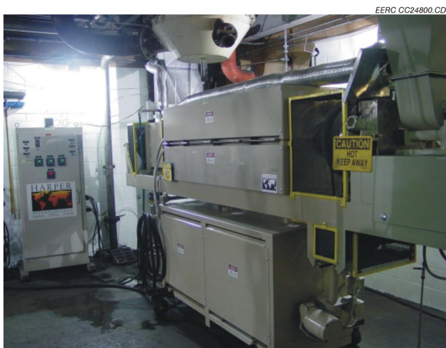
Figure 4. The rotary kiln reactor system installed in the EERC pilot plant.
