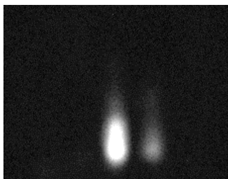
Figure 4. Native PAGE gel image showing chemiluminescent signal from A. cryptum JF-5 protein extracts. Chemiluminescence is produced where proteins are reducing Cr(VI) to Cr(III).
