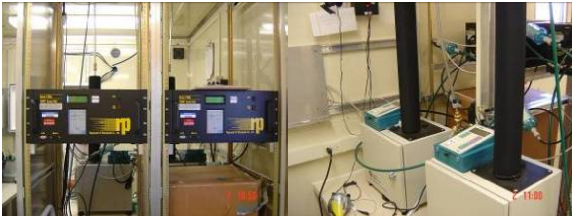
Figure 7. Left photograph: The front panels of PM 10 (right on the left photograph) and PM 2.5 (left on the left photograph) of TEOM. Right photograph: The DUSTTRAK monitors (green) resting on top of the two TEOM measuring units
