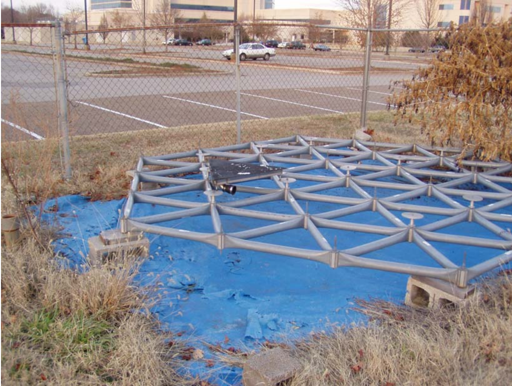
Figure 2 – Geometrica Tower Reflector Support Structure with Tower Reflector Facet at University of Alabama in Huntsville
