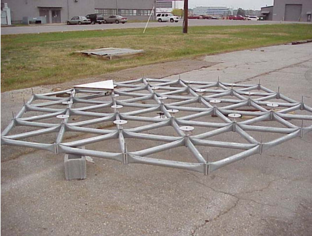
Figure 6 - Geometrica Geodesic Dome Support Structure Test Article, with Tower Reflector Facet
