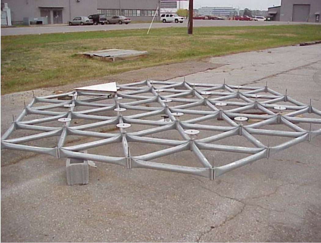
Figure 1 – Geometrica Tower Reflector Support Structure with Tower Reflector Facet at NASA MSFC
