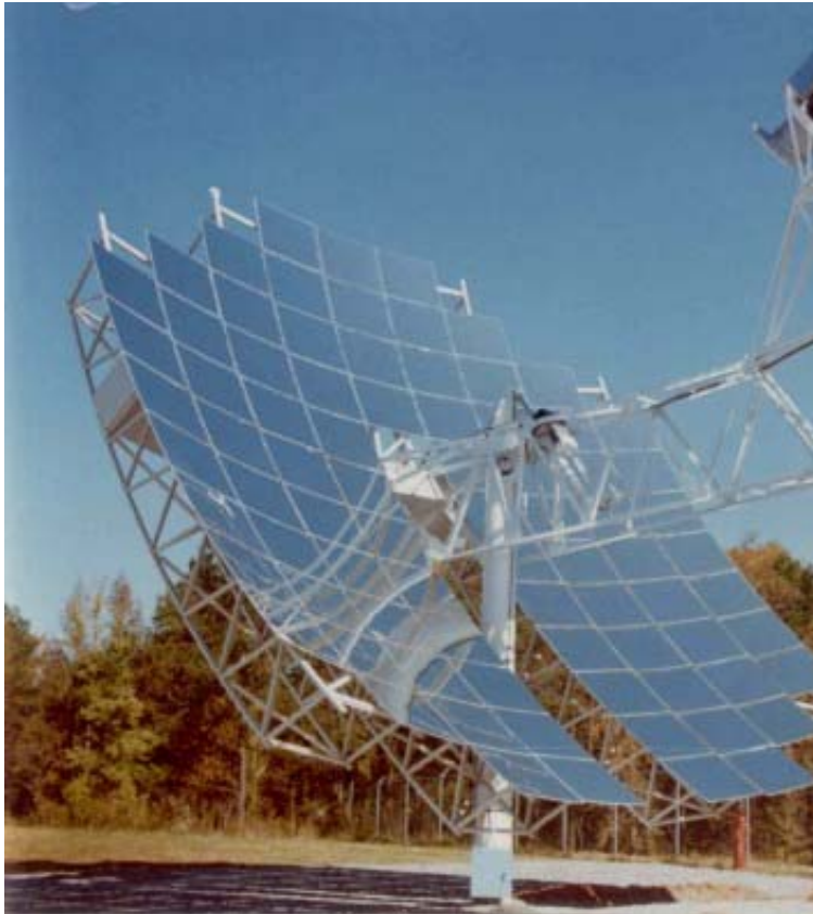
Stirling Energy Systems 25 Kilowatt Electric Dish Stirling Solar Power System Concentrator – World's record for net solar electric efficiency Available) in the field (Developed by McDonnell Douglas, 1982-1984)
