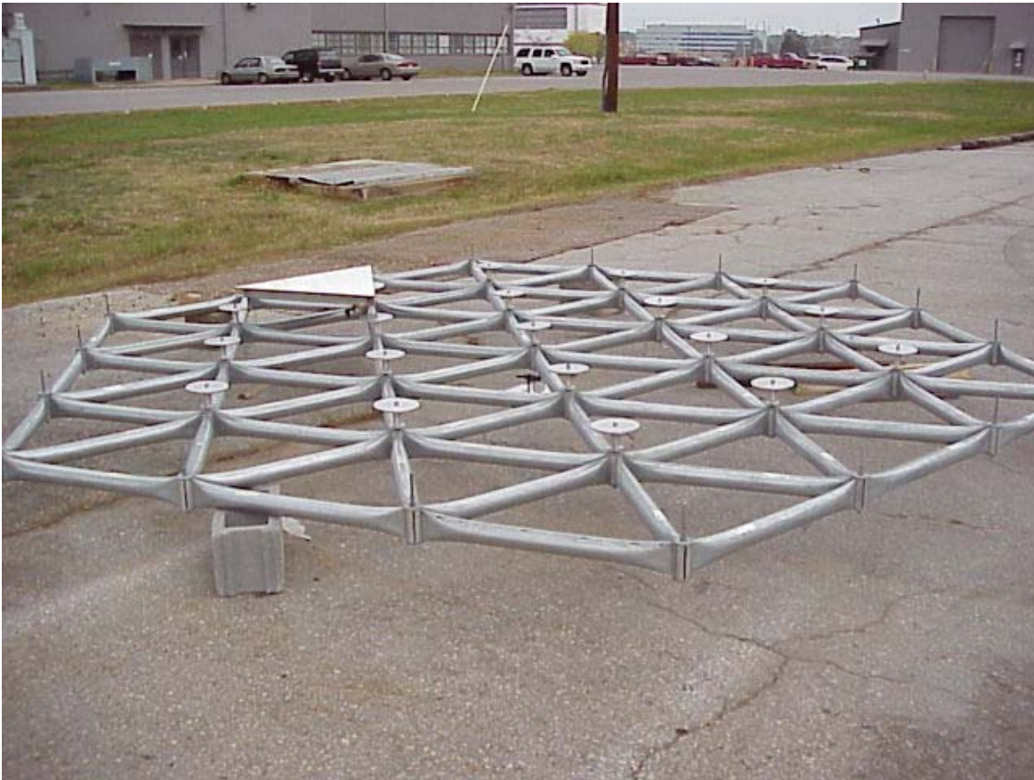
Geometrica Geodesic Dome Support Structure Test Article, with Tower Reflector Facet
