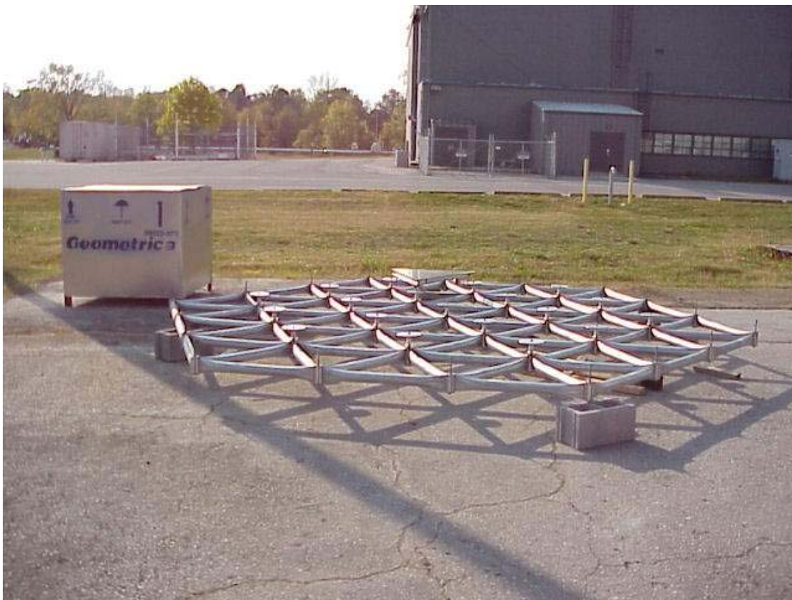
Figure 4 – Geometrica Structure with Tower Reflector Facet Undergoing Long Term Exposure Test at NASA MSFC
