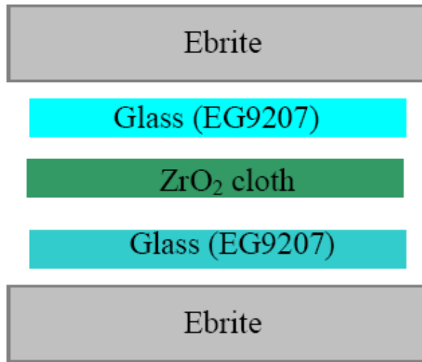
Figure 3.42 Sample configuration to examine evolution of glass in air
