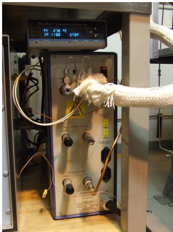
Figure 3.57 Steam injection humidifier for wet hydrogen contact resistance testing.
