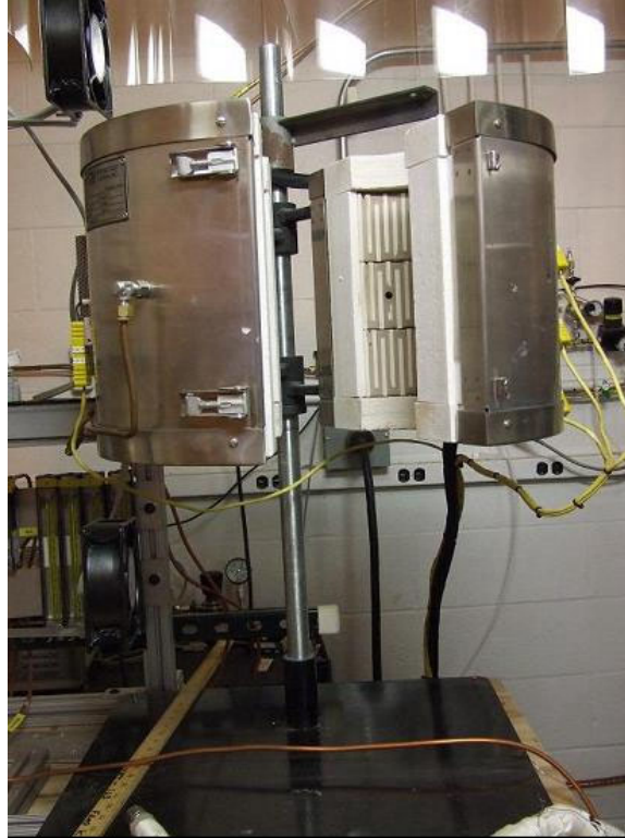
Figure 3.56 High temperature furnace for wet hydrogen contact resistance testing.
