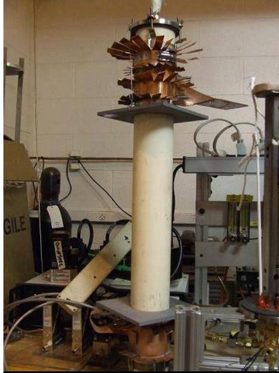
Figure 3.55 Alumina support tube for wet hydrogen contact resistance testing.
