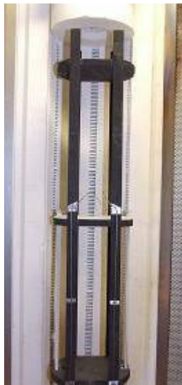
a) b) Figure 3.53 Test setup for off-line ASR testing. a) Test stand that can accommodate 6 samples (2 per level). b) A single level showing thermocouples and electrical connections.
