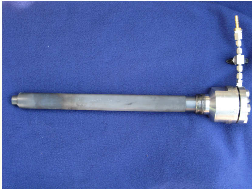
Fig.G4.6 After first rig test of probe, expected part frontend discoloration is seen due to chemical exposure in combustor refractory section.
