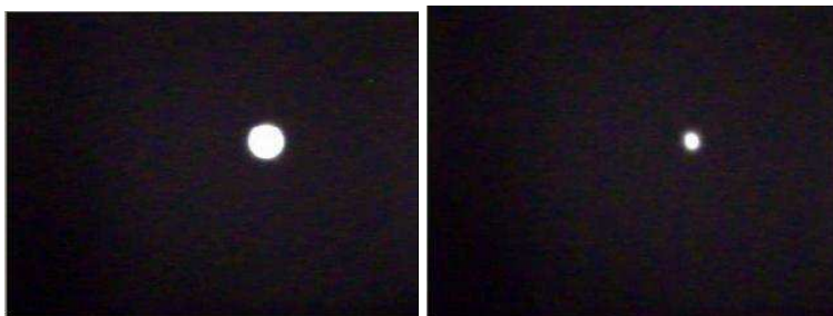
Fig.G4.5. IR CCD camera (8.8 mm x 6.6 mm active area view) received laser beam snap shots during thermal shock stage indicating on/off oscillatory Fabry-Perot etalon behavior of SiC optical chip due to the rapid thermal gradient. Left Photo: Power Max; Right Photo: Power Min.
