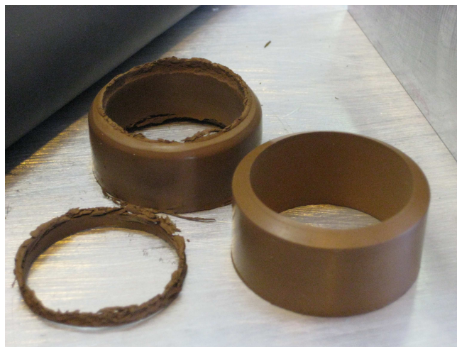
Fig.G4.13. Condition of Viton seal used in the probe connector before and after 28 days in rig.
