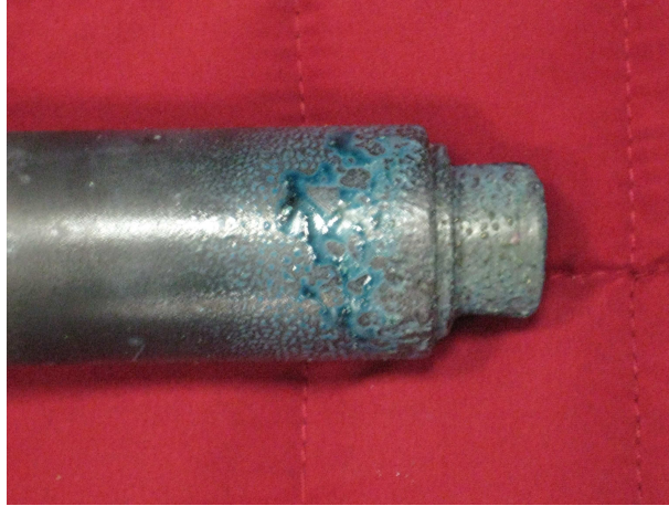
Fig.G4.14 Probe condition showing copper sulphate deposits after 28 continuous days in the rig.
