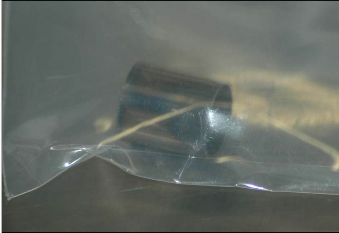
Figure 4.15. Control Sample Zy11 Heated for 12.5 hours at 546°C.
