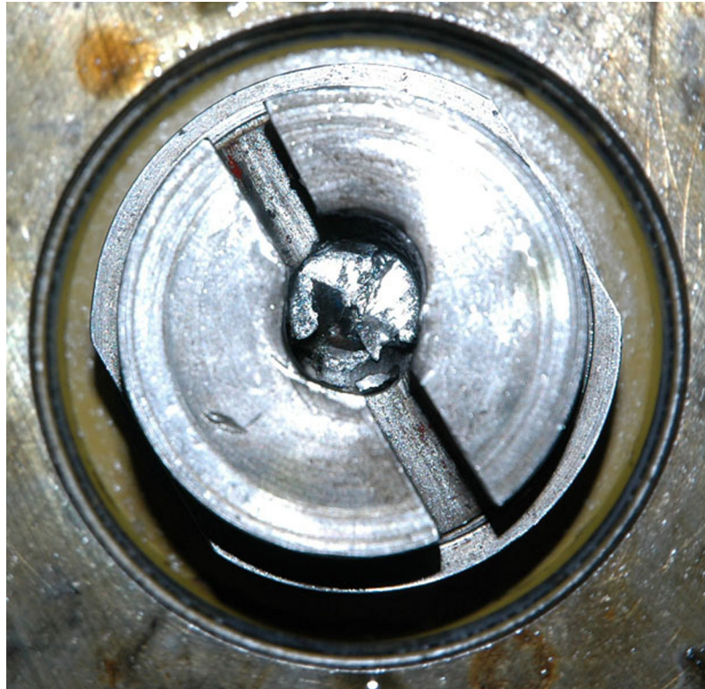
Figure 4.1. Press ram locking mechanism, damaged after HX-1.
