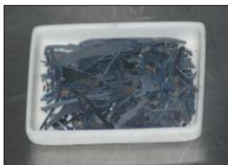
(a) ZrH 2 shards produced at ~540°C
