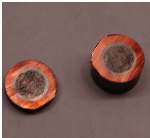
Figure 4.2. Sectioned HX-1 billet, unextruded. Copper canister, Zircaloy sheath, and cermet mixture visible.
