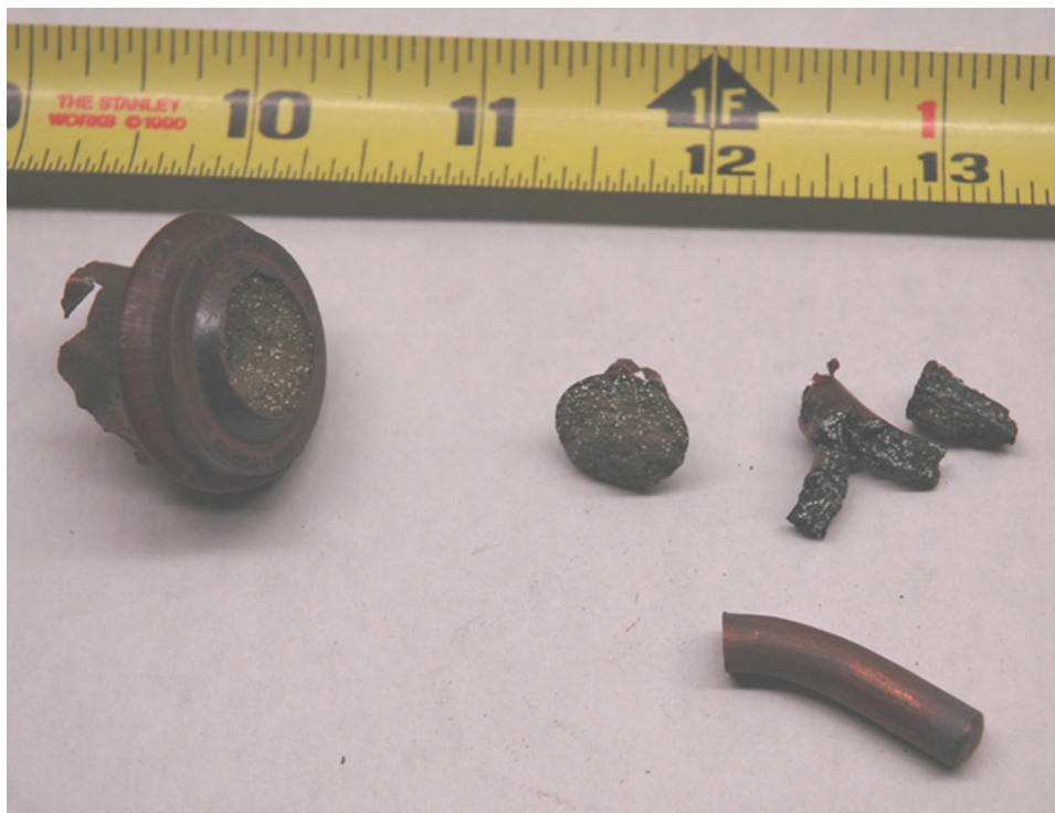
Figure 4.9. Remnants of HX-6, showing copper extrusion, burst, and remaining billet. Smaller sections
