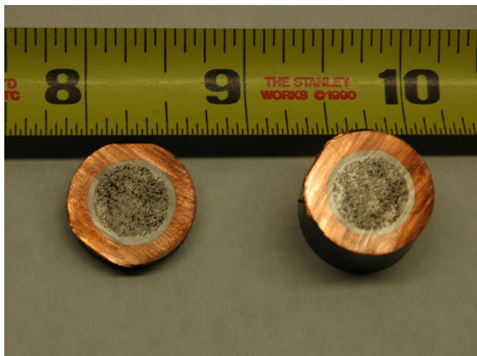
Figure 4.4. Sectioned billet from HX-2, unextruded. Copper canister, Zircaloy tube, and cermet powders visible
