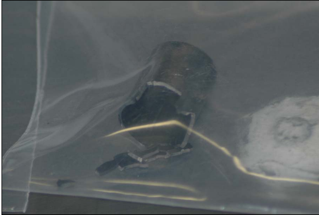
Figure 4.14. Sample Zy10 after Hydriding for 3 hours at \sim 543^{\circ}\text{C} and 3 hours at \sim 383^{\circ}\text{C} .
