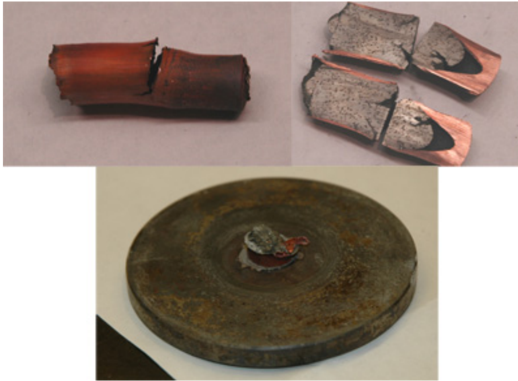
Figure 4.14. Extrusion experiment HX-8 results showing die, extruded billet, and sectioned billet.
