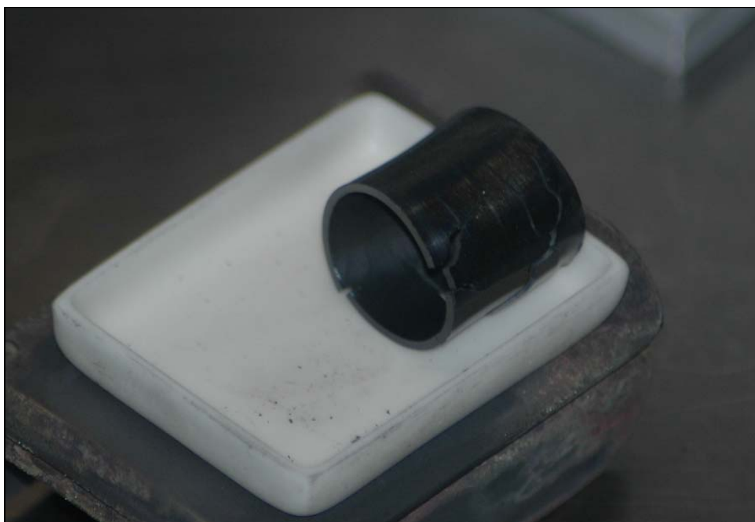
Figure 4.19. Sample Zy14 after Hydriding for 8 hours at ~539°C.
