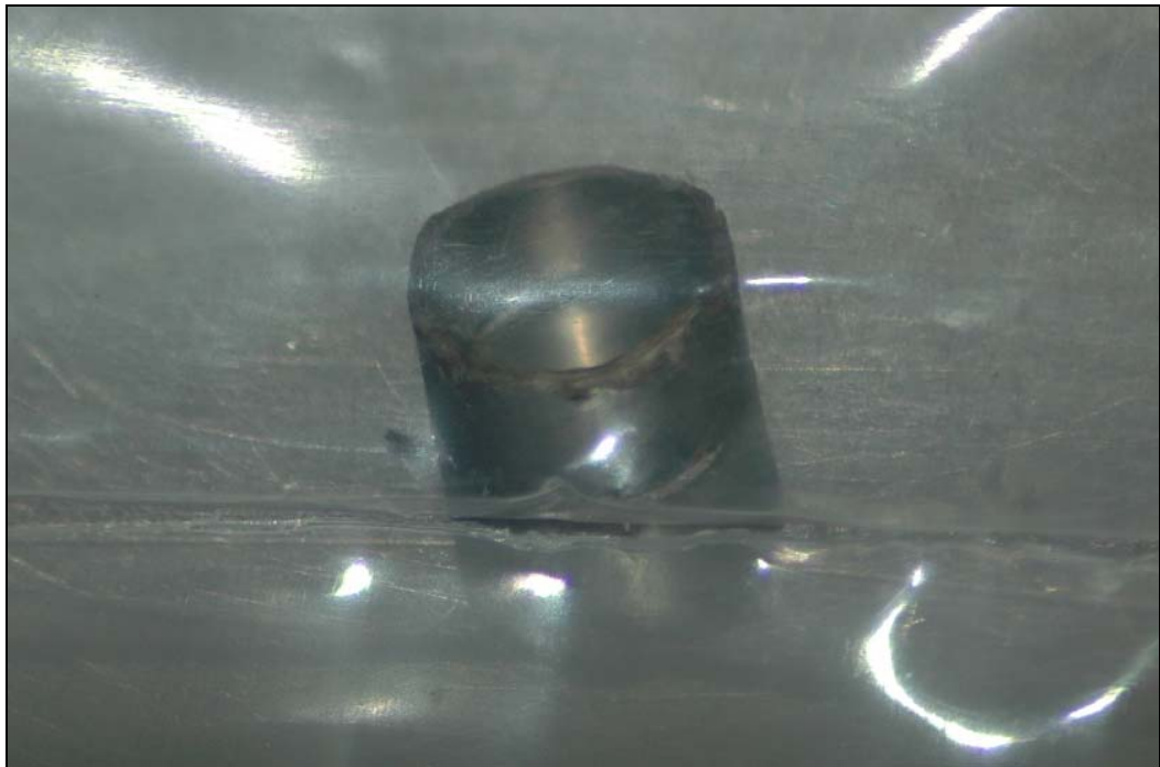
Figure 4.4. Sample Zy1 After Hydriding for 6 hours at ~360°C.
