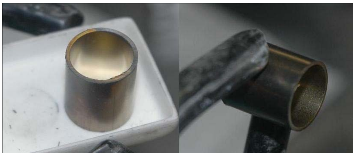
Figure 8. Golden color of experiment 24 indicating nitride contamination.
