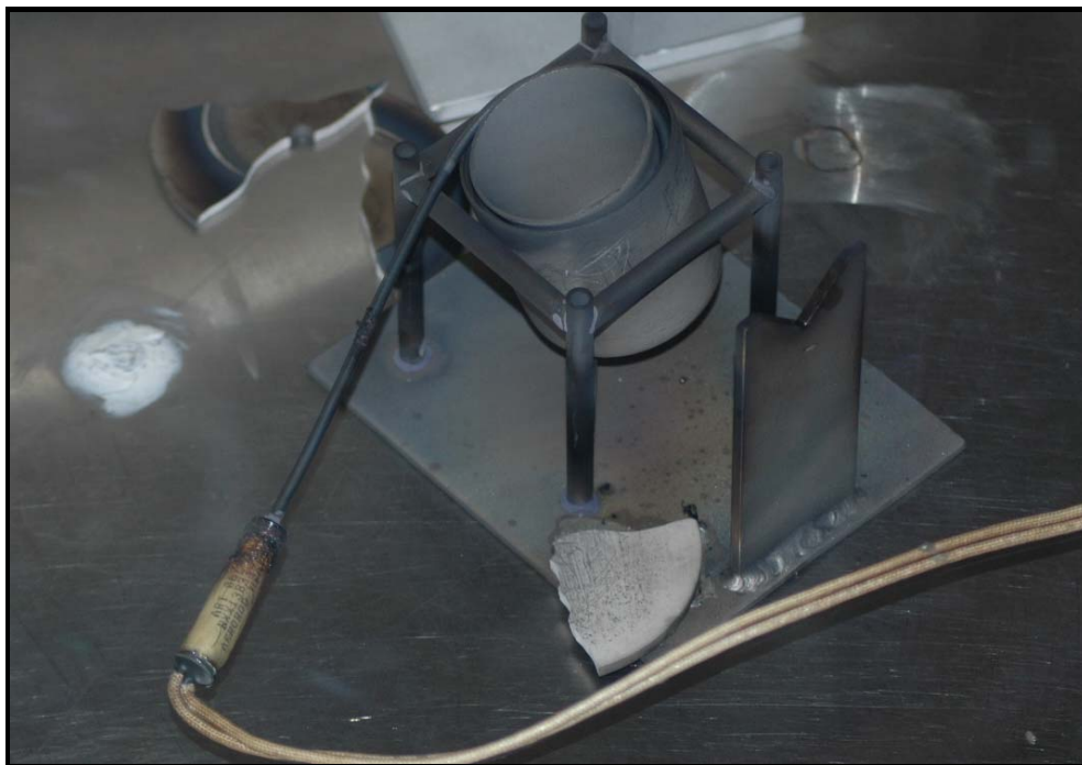
Figure 4.24. Dehydride Apparatus After the Calibration Run and Heater Failure.
