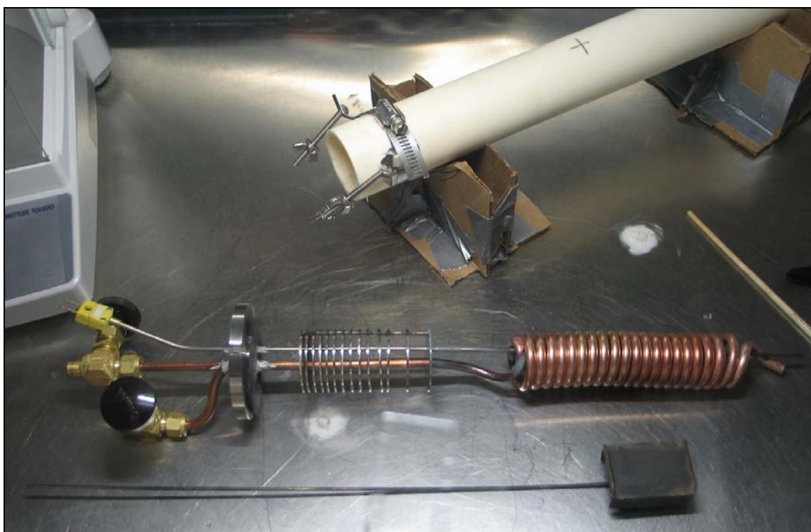
Figure 3.3. Photo of the Hydride Reaction Vessel Showing the Alumina Tube, the Tube Seal and the Sample Tray.
