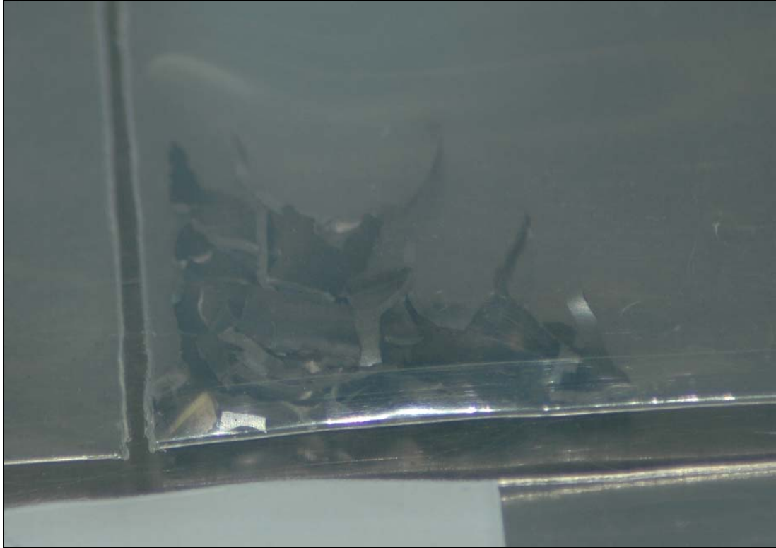
Figure 4.11. Sample Zy7 after Hydriding for 24 hours at \sim 525^{\circ}\text{C} .
