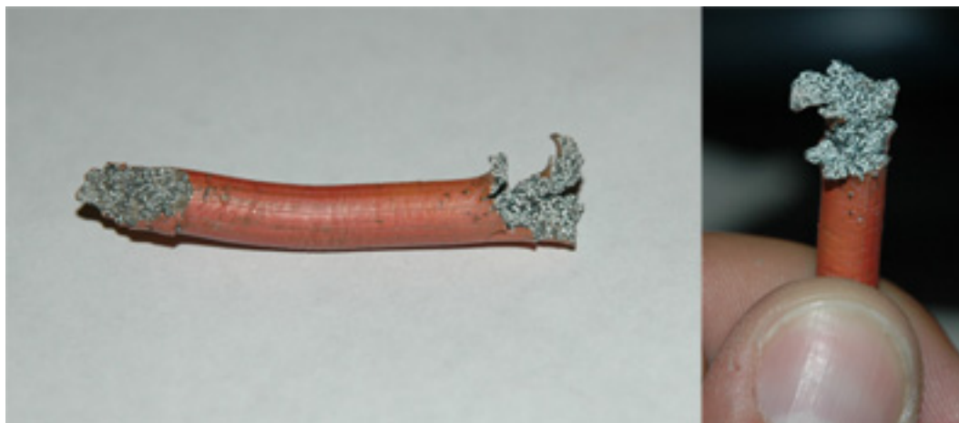
Figure 4.12. Damage in HX-7. Left: full rod, showing break at beginning and end of cermet. Right: closeup of rod burst.
