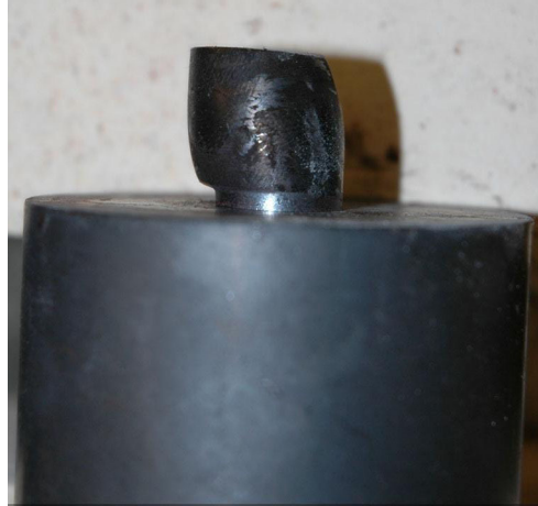
Figure 4.3. H-13 tool steel extrusion ram destruction after HX-2.
