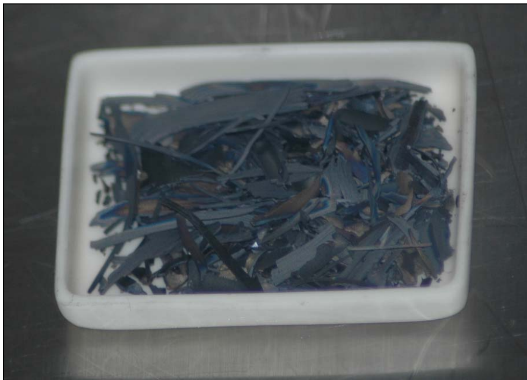
Figure 4.9. Sample Zy5 after Hydriding for 12 hours at \sim 503^{\circ}\text{C} .
