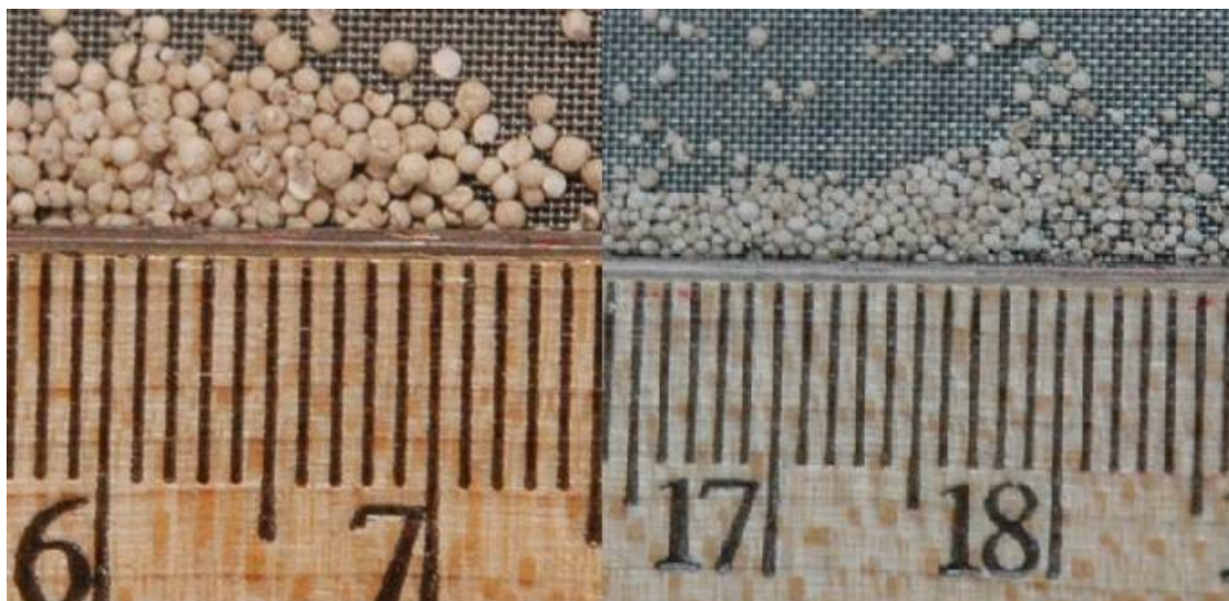
Figure 30. Photo of experiment 70 product; non-heated on left and sintered on right.
