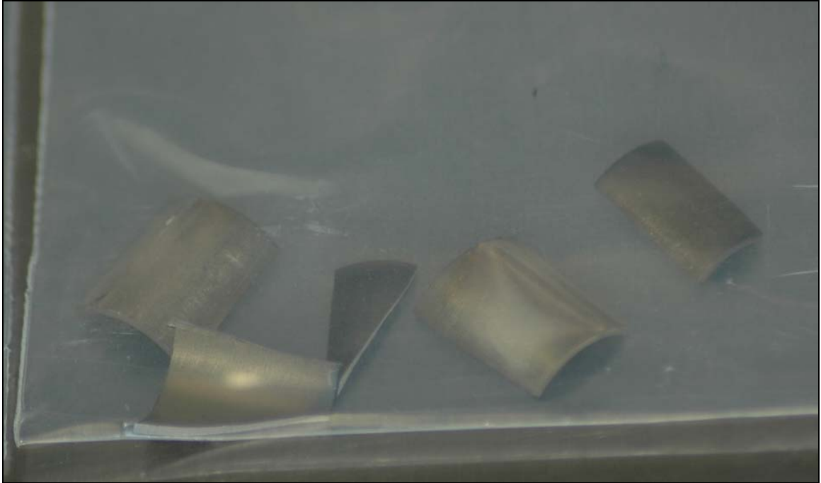
Figure 4.16. Sample Zy12 after Hydriding for 5.2 hours at \sim 755^{\circ}\text{C} .
