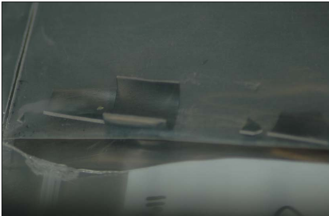
Figure 4.5. Sample Zy2 after Hydriding for 6 hours at ~733°C.
