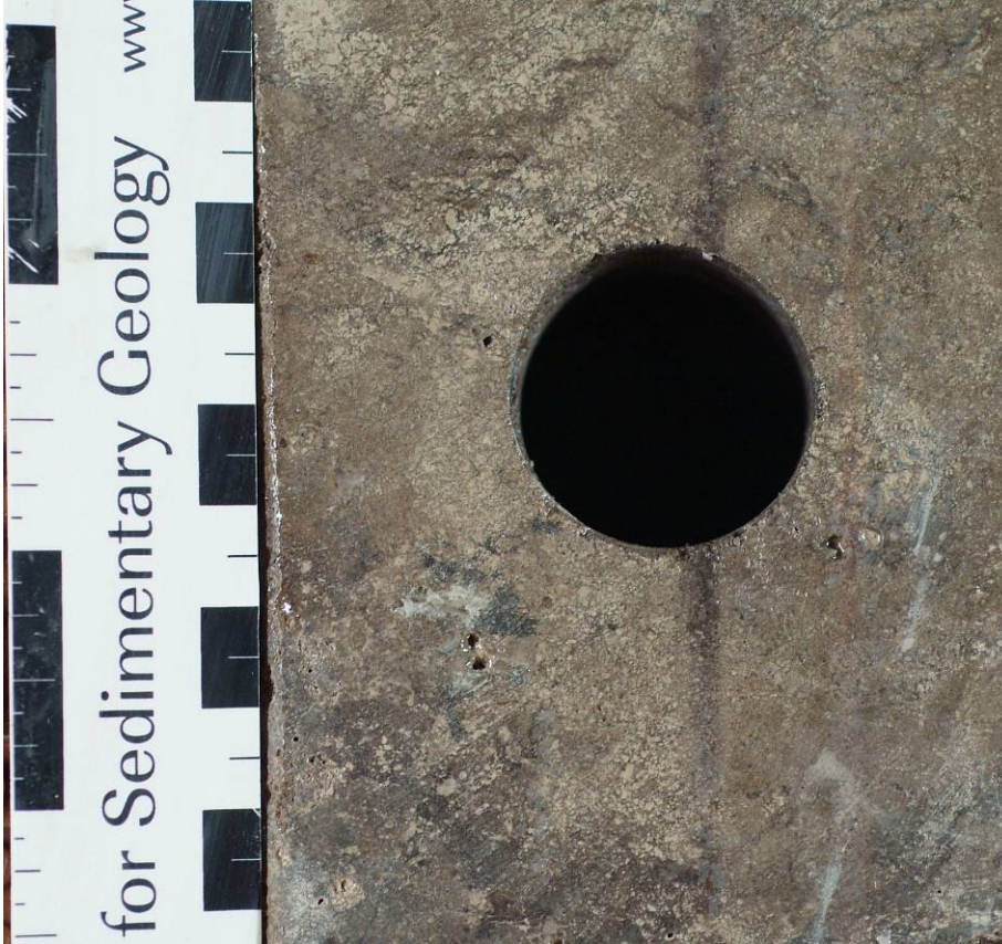
Figure 55. Core photograph from petrophysical facies P-4 with only small vugs visible. Charlton (4710 ft.)
