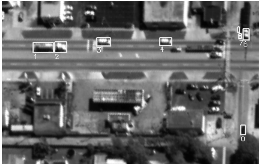
Figure 4: Newly initialized tracks shown with initial bounding boxes and track ID's
