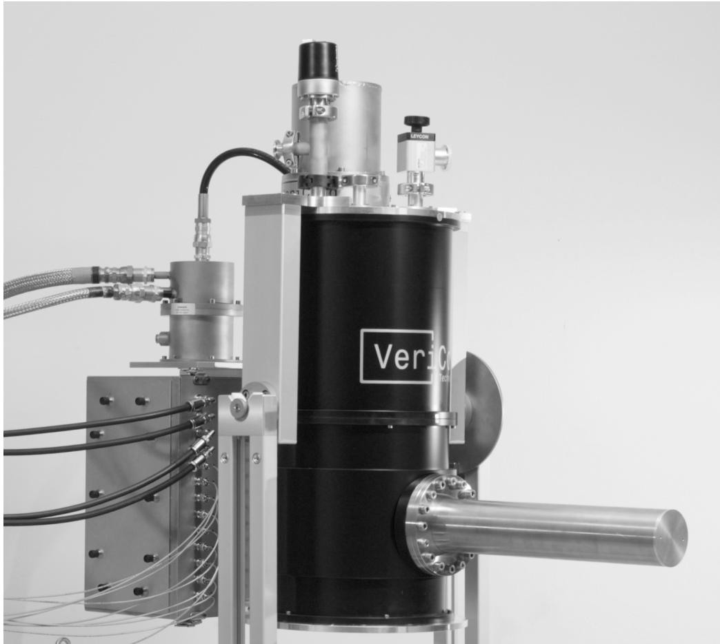
Figure 1: Photograph of the pulse-tube ADR. The STJ detector is held at the end of the cold finger, and the preamplifiers are located in the shielded enclosure on the opposite side. The rotary valve (in the back) between the pulse tube and the compressor is mechanically and electrically isolated from the main body of the instrument.
