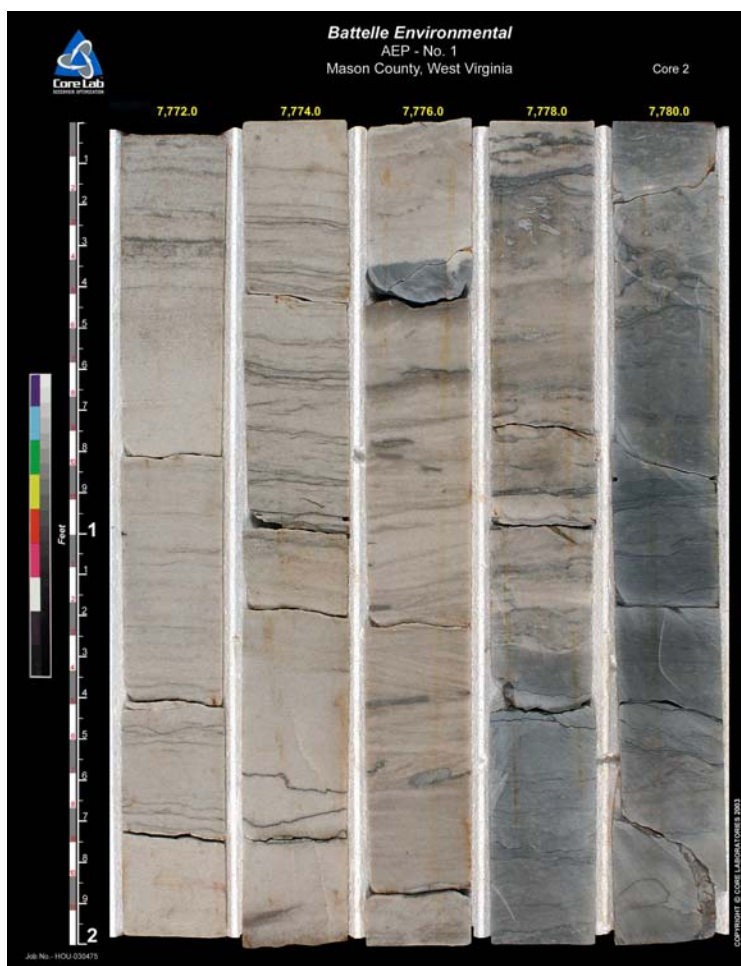
Figure 3-8. Example of 3-Inch Diameter Continuous Core (This Core was Collected From the Rose Run Sandstone at a Depth Interval of 7,772 to 7,782 ft.)
