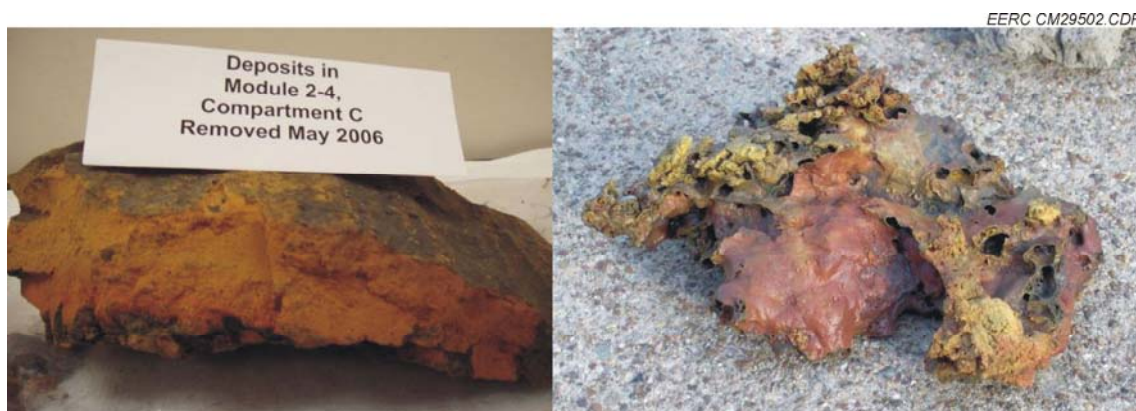
Figure 44. Photos of representative deposit samples collected from Hopper C. On the left is a sample of the monolithic deposit, and on the right is a sample of the hard popcorn deposit that has been rinsed. Images are not to the same scale.
