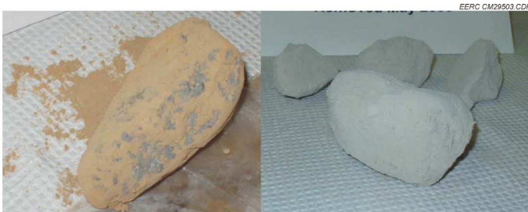
Figure 46. Photos of representative deposit samples collected from Hopper H: the sample on the left is referred to as the “orange” deposit, and those on the right are the “gray” deposits. Images are not to the same scale.
