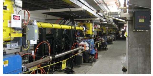
Figure 3. LER vacuum chamber in IR12 (upper beam pipe). The outer clearing solenoid can be seen.
