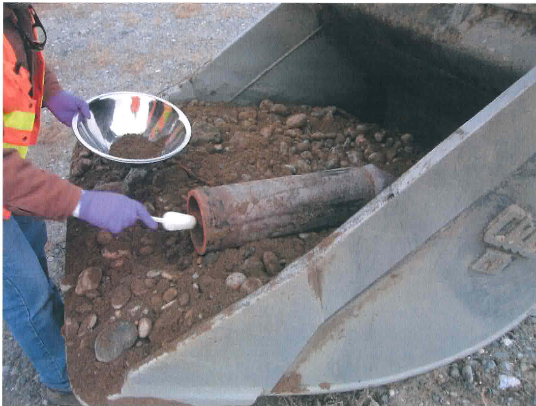
Photograph A-8. Sampling of Vitrified Clay Pipe from Test Pit 3 (December 2006).
