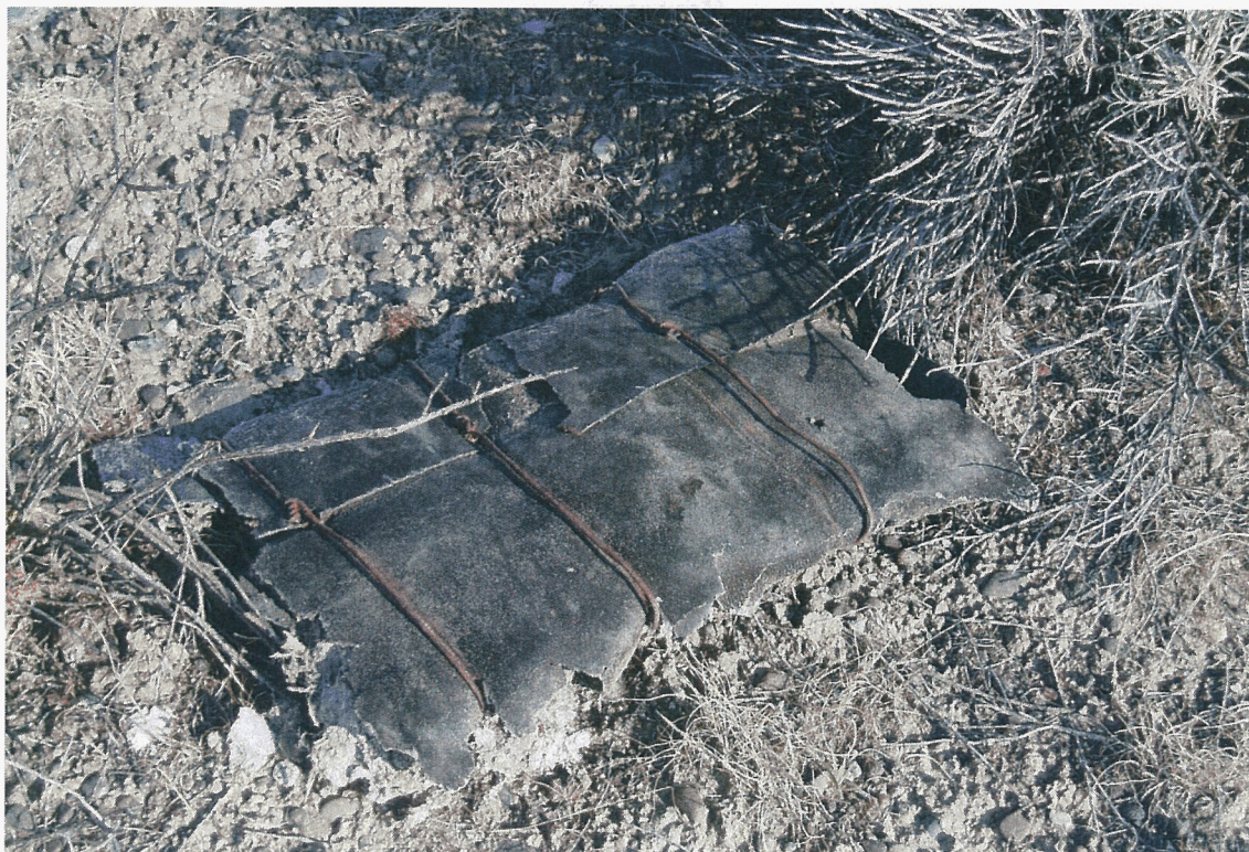
Figure A-2. Photograph of Potential Friable ACM Material (Pipe Wrapping – ID #5).
