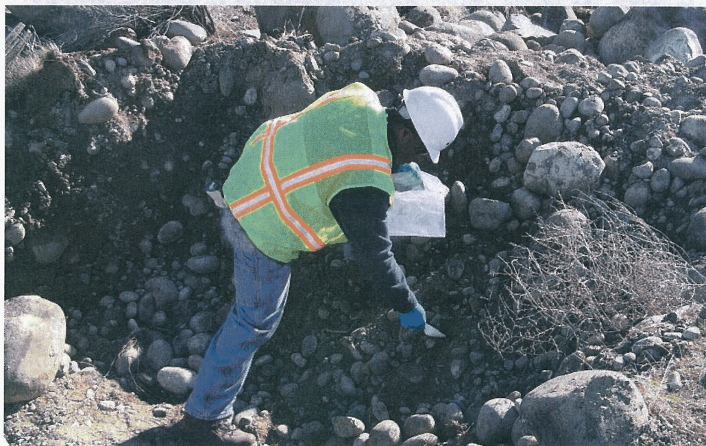
Figure A-8. Stained Soil Underlying Leaking Battery Cache (ID #85).
